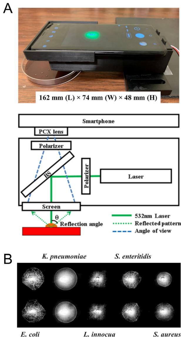
Fig. 24 Smartphone imaging and identification of bacterial colonies via elastic light scattering and machine learning. (A) Design of the smartphone-based device. (B) Examples of backscatter patterns from colonies of several species of bacteria. Abbreviations: BS, beam splitter; PCX, Plano-convex. Figure reproduced from ref. 399 under a Creative Commons CC BY 4.0 licence.
