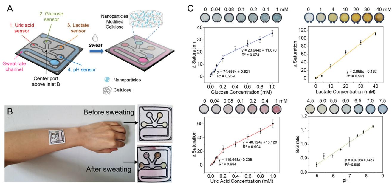
**Fig. 50** Wearable  $\mu\text{PAD}$  for the analysis of sweat biomarkers: uric acid, glucose, lactate and pH. (A) Design of the  $\mu\text{PAD}$ . The NP detection region is highlighted. (B) After sweat exposure, a color change is visualized. (C) Calibration curves (based on HSV color saturation (S) or a B/G channel ratio) for the analytes from smartphone imaging of the  $\mu\text{PAD}$ . Adapted with permission from ref. 573 Copyright 2023 Wiley-VCH GmbH.
