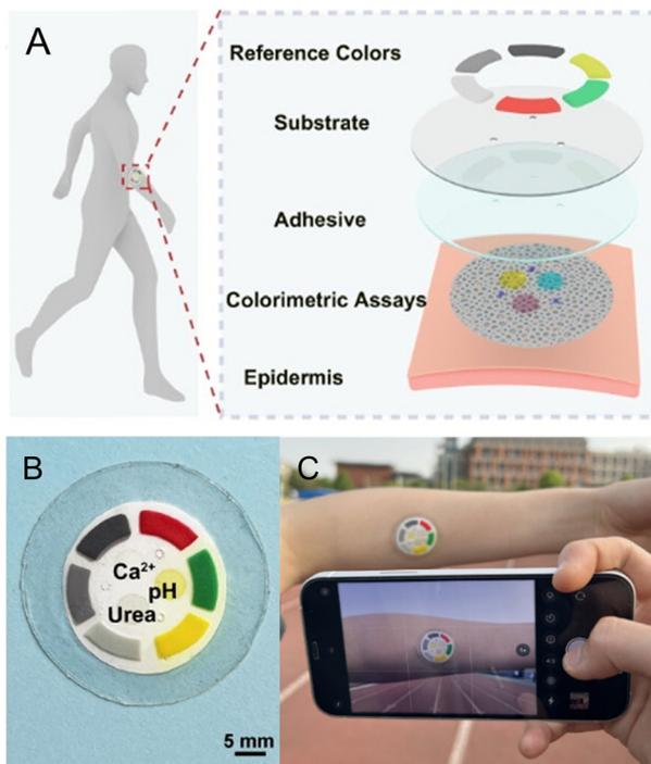
**Fig. 17** Stretchable patch for colorimetric sweat sensing directly from skin. (A) Design of the patch. (B) Photograph of the patch with six reference colors and indicator spots for detecting pH, urea, and Ca<sup>2+</sup> (aq). (C) Smartphone imaging of the patch for *in situ* colorimetric analysis. Adapted with permission from ref. 164 Copyright 2024 American Chemical Society.
