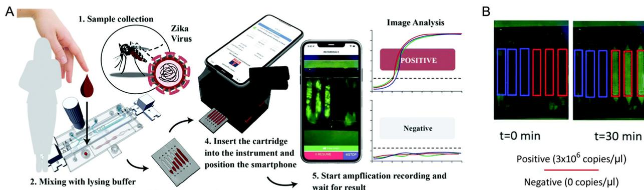
**Fig. 48** Point-of-care blood testing for Zika virus with smartphone-based detection. (A) Assay workflow with a multi-stage manually actuated microfluidic chip for sample processing and transfer to a detection cartridge for smartphone-based fluorescence imaging. (B) Smartphone images for in-cartridge detection of virus spiked into whole blood. Adapted from ref. 460 Copyright 2022 The Royal Society of Chemistry.
