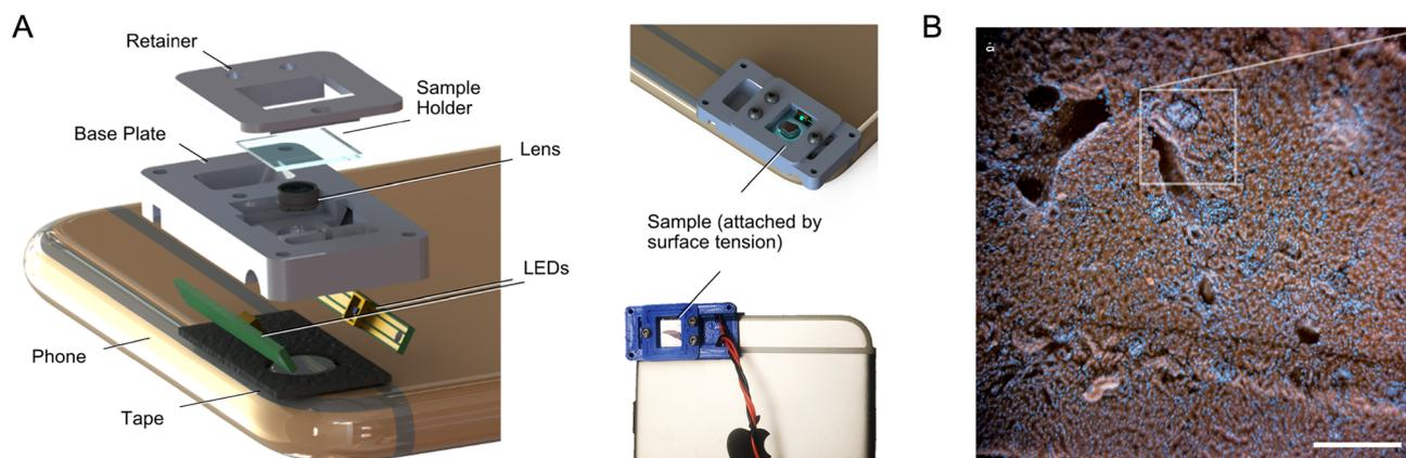
**Fig. 33** Compact smartphone mounted microscope. (A) Design of the microscope attachment, which uses ultraviolet surface excitation. (B) Fluorescence image of a mouse kidney section stained with rhodamine B and DAPI dyes. Figure adapted from ref. 483 under a Creative Commons CC BY 4.0 license.
