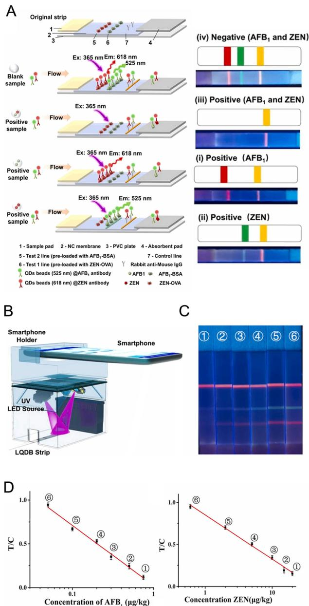
**Fig. 27** Two-color, two-line multiplexed competitive LFIA with fluorescence detection. (A) Assay design and smartphone images of assay outcomes. (B) Design of the smartphone-based device used to image the LFIAs. (C) Smartphone images of LFIAs and (D) the corresponding calibration curves for each analyte, aflatoxin B1 (AFB1) and zearalenone (ZEN). The y-axis in panel D is the ratio of signal between the test and control lines. Adapted from ref. 78 with permission from Elsevier.
