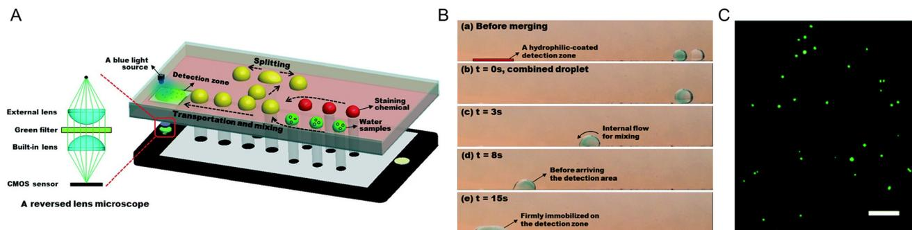
**Fig. 47** Smartphone display-actuated optoelectrowetting droplet microfluidics for on-chip sample preparation and water quality detection. (A) Schematic overview of the digital microfluidic operations and (B) video frames showing these operations. (C) Smartphone-acquired fluorescent image of marine water sample showing target algae cells. The scale bar is 100  $\mu\text{m}$ . Adapted from ref. 568 Copyright 2018 Royal Society of Chemistry.
