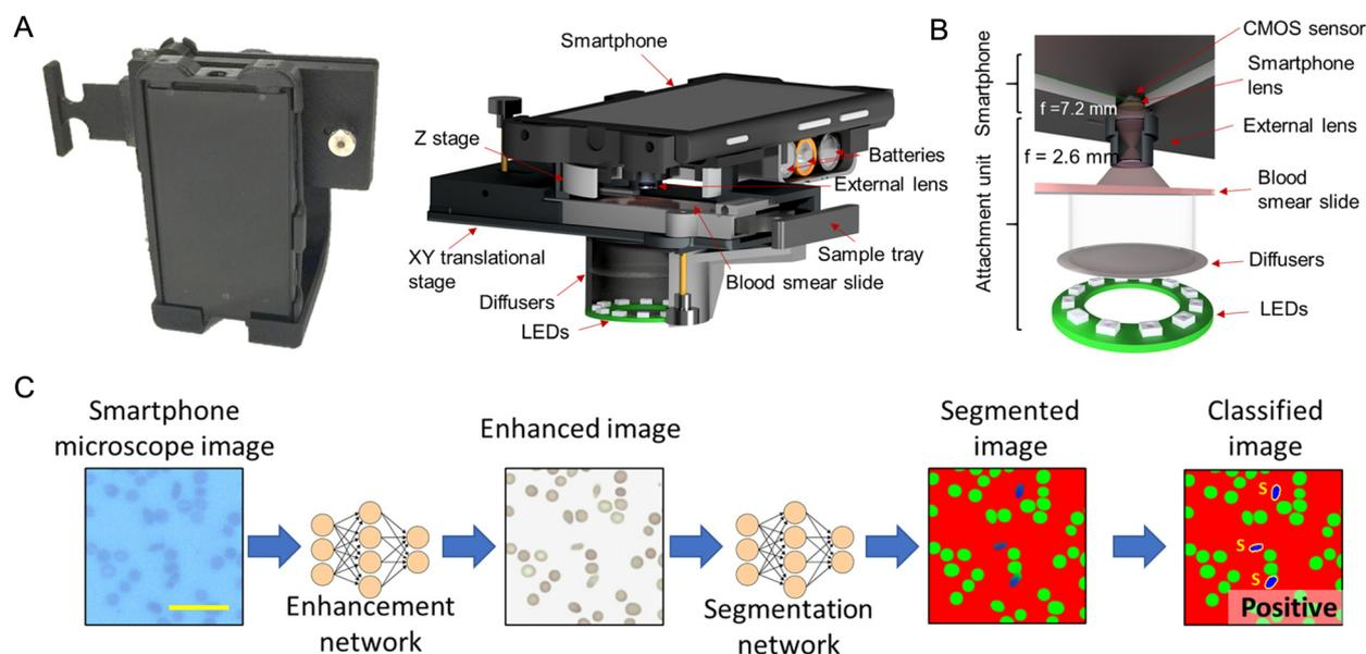
**Fig. 23** Smartphone-based brightfield microscope for sickle cell identification. (A) Photograph (left) and design (right) of the microscope device. (B) Close-up of the optical path. (C) Workflow from image acquisition to identification of sickle cells. Adapted from ref. 89 under a Creative Commons Attribution 4.0 International License.
