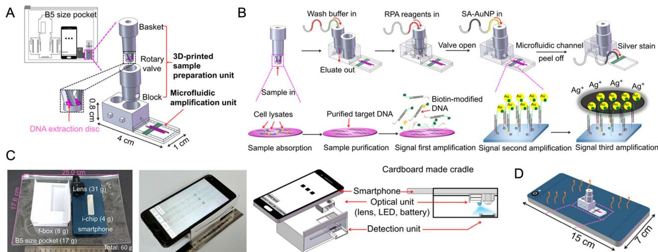
**Fig. 49** Smartphone-based colorimetric detection of target DNA sequences using a pocket-sized basket-and-microfluidic system for sample preparation and assay execution with a foldable box. (A) Design of the device. (B) Assay workflow. (C) Photographs of the smartphone-based foldable-box device. (D) Illustration of how the smartphone is used to provide heat for DNA amplification. Figure adapted from ref. 571 under a Creative Commons CC BY 4.0 license.
