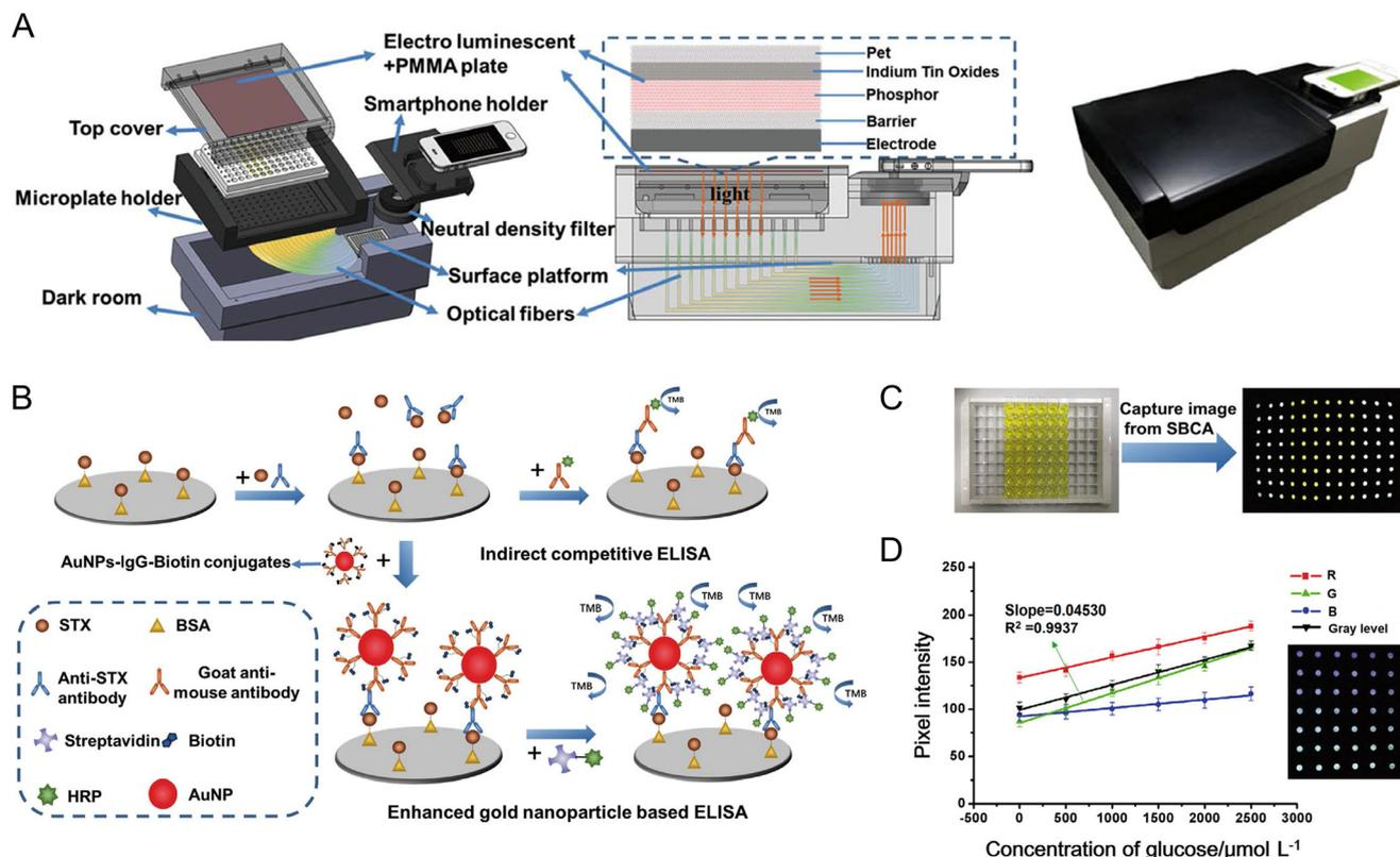
**Fig. 16** Smartphone-based colorimetric analyzer for an AuNP-enhanced ELISA. (A) Device design. (B) Assay method. (C) Smartphone image (right) derived from the multi-well plate (left). (D) Plot of pixel intensity versus glucose concentration from RGB and grayscale image analysis. Abbreviations: STX, saxitoxin; BSA, bovine serum albumin. Also refer to the Abbreviations list. Adapted with permission from ref. 278 Copyright 2019 Springer Nature.
