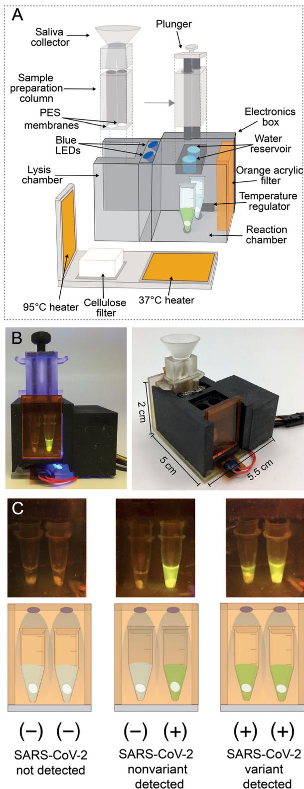
**Fig. 30** Sample-to-answer device for CRISPR-based detection SARS-CoV-2 and variant nucleic acids. (A) Design of the device, including sample processing (left) and assay (right) modules. (B) Photographs of the device, which is capable of two-plex detection. (C) Smartphone-acquired fluorescence images of samples. Figure reproduced from ref. 470 under a Creative Commons CC BY 4.0 license.
