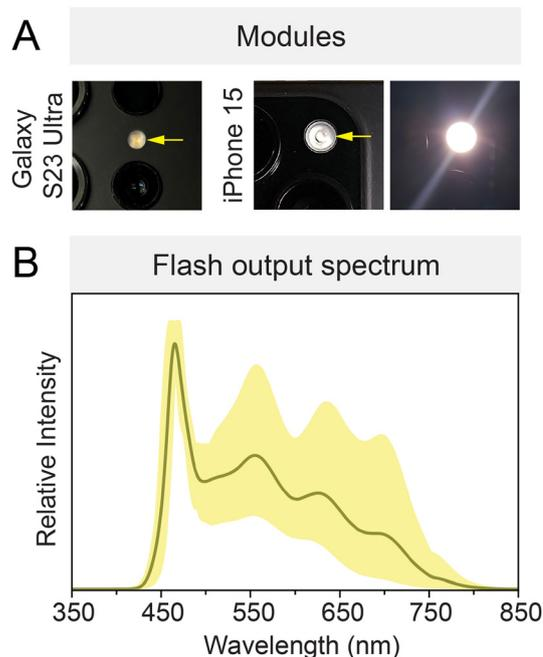
**Fig. 3** Smartphone flashlight (or torch). (A) Examples of the exterior view of smartphone flashlight modules (marked with arrows). (B) Typical flashlight output spectrum. The solid line in panel B represents the average output spectrum from the flash across 18 different models and 3 manufacturers of smartphones; the shaded regions reflect the highest and lowest output at a given wavelength. The data in panel B was measured for this review.
