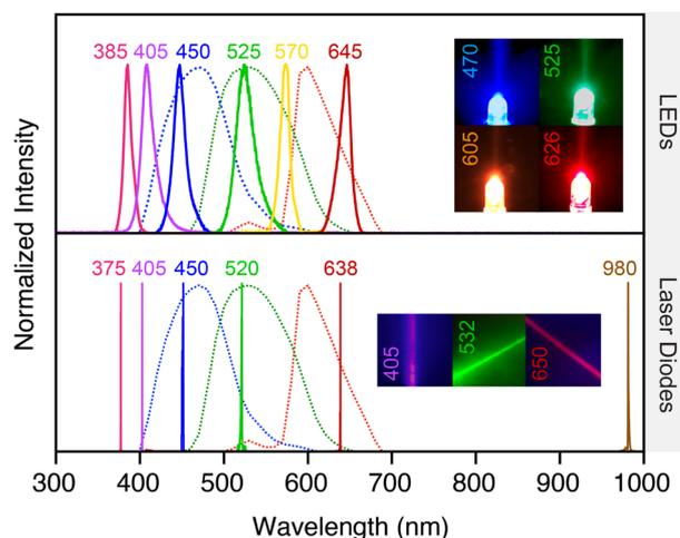
**Fig. 5** LEDs and laser diodes. Examples of emission spectra of LEDs (top) and laser diodes (bottom) superimposed on the average spectral responses of the smartphone camera RGB color channels (dotted lines). The insets show images of LEDs and beams from laser diodes. Some digital adjustment of color was made to these images to mimic the appearance to the human eye. LED and laser diode spectra were plotted from publicly available vendor data (ThorLabs) for commercial products.
