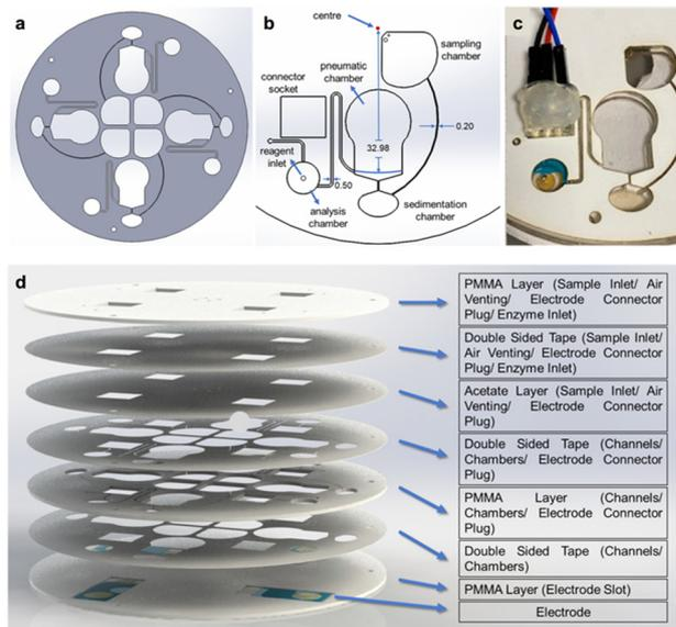
**Fig. 1** The design and the fabrication process of the cartridge used in the lab-on-a-CD system. The cartridge design (a), dimensions of the components (b), their installation on the CD (c), and layers of the disc (d) are illustrated and described.
