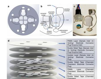
Fig. 1 The design and the fabrication process of the cartridge used in the lab-on-a-CD system. The cartridge design (a), dimensions of the components (b), their installation on the CD (c), and layers of the disc (d) are illustrated and described.
