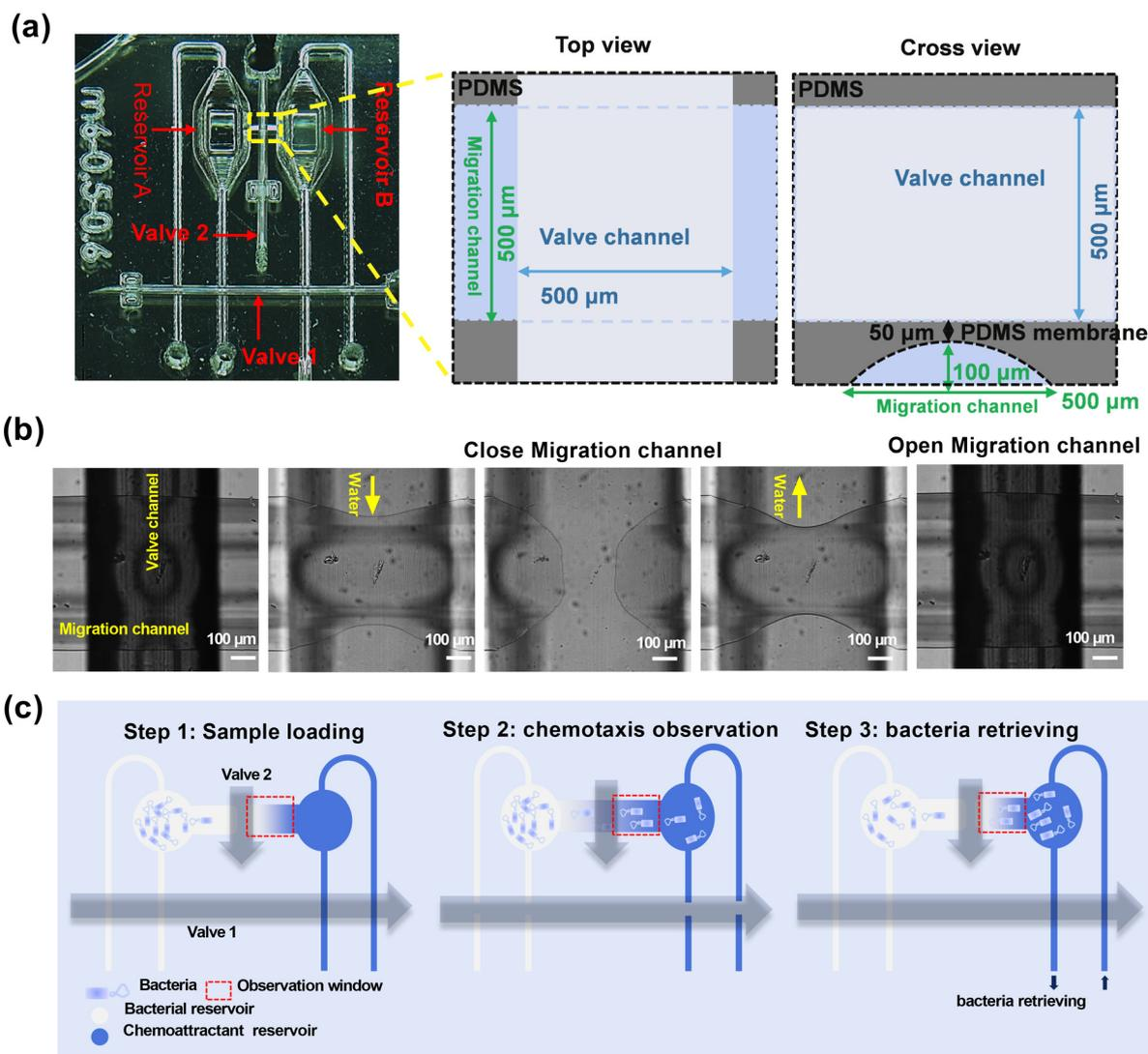
**Fig. 1** Microfluidic chip design. (a) Optical image of the chemotaxis microfluidics device. Zoom-in pictures of two on-chip valves controlling on/off of the migration and delivery channels. (b) Time-lapse images showing valve 2 opening and closing the migration channel. (c) Operation steps for studying and sorting chemotactic cells. By controlling the valve channels, this system enables *in situ* observation of chemotaxis and simultaneous isolation of chemotactic bacteria.
