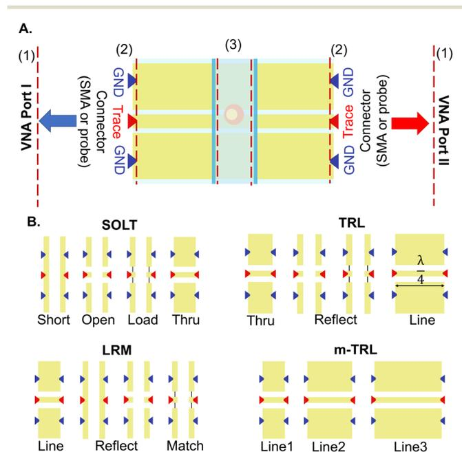
**Fig. 6** Overview of the calibration technique. A) Two steps of calibration to move reference planes (shown with dashed red lines) from VNA ports (1) to connector tips (2) followed by a de-embedding step to move them further to the sample (3). B) Calibration standards on-chip. Arrows represent the placement of on wafer probes.
