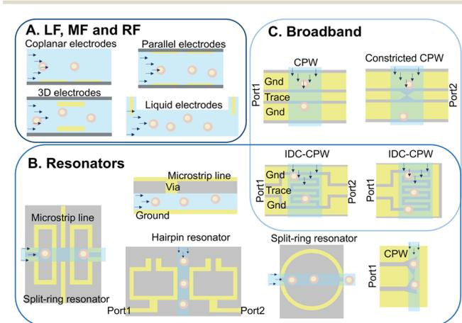
**Fig. 4** Examples of different electrode configurations used in IDS cell characterisation at low frequency (kHz–MHz) (A), broadband (kHz–GHz) (B) and narrow-band (GHz) (C) setups. Cells can be suspended or cultured in the sensing area, however, here they are flowing through the channels.
