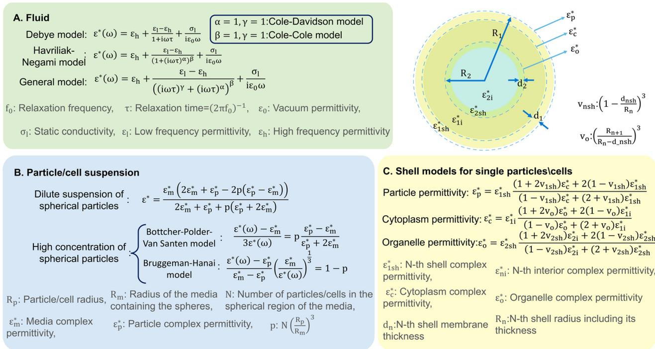
**Fig. 2** A graphical representation depicting various analytical models developed for analysing A) liquids, B) particle or cell suspensions in liquids, and C) single cells or particles in a liquid.
