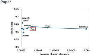
Fig. 3 Mesh convergence test. Parameters of the micromixer with parallelogram barriers:  $\alpha$  = 45 deg, l = 250  $\mu$ m, p = 500  $\mu$ m, d = 1500  $\mu$ m, and Re = 1.
