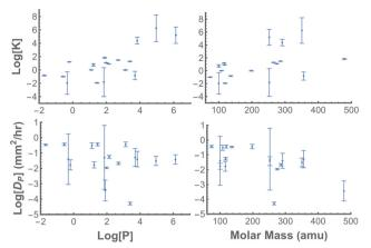
Fig. 7 Correlations of PDMS-interaction parameters with select chemical properties. (Top) The PDMS-water partition coefficient ( $\log K$ ) generally increases with increasing  $\log P$ , i.e. increasing hydrophobicity, and with increasing molar mass. No relationship is observed with H-bond donor count. (Bottom) Diffusivity in PDMS ( $\log D_P$ ) generally decreases with increasing molar mass. No relationship is observed with  $\log P$  or H-bond donor count.
