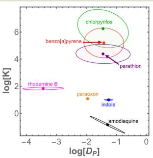
Fig. 4 Fitted values of  $\log D_P$  and  $\log K_{PW}$  with corresponding error ellipses for four chemicals measured directly in aqueous solutions (amodiaguine, indole, paratoxon, rhodamine B) and three measured in solutions with DMSO (benzo[a]pyrene, chlorpyrifos, and parathion).
