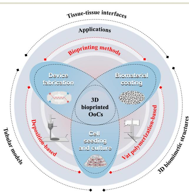
**Fig. 1** A schematic illustration of 3D bioprinted organs-on-chips (OoCs). OoCs can be directly fabricated by 3D bioprinting techniques including deposition-based and vat polymerization-based bioprinting, which enhance the structural and functional fidelity of organ models and broaden the applications of OoCs.
