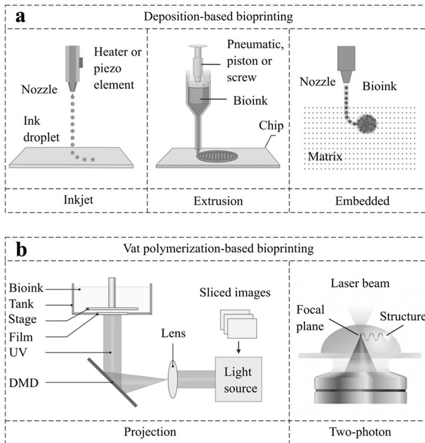
**Fig. 3** Bioprinting strategies used in OoCs. (a) Schematic illustration of the deposition-based bioprinting technique, which contains inkjet-, extrusion-, and embedded-based approaches for depositing bioinks. (b) Schematic illustration of the vat polymerization-based bioprinting technique, which contains projection- and two-photon-based approaches for shaping bioinks.
