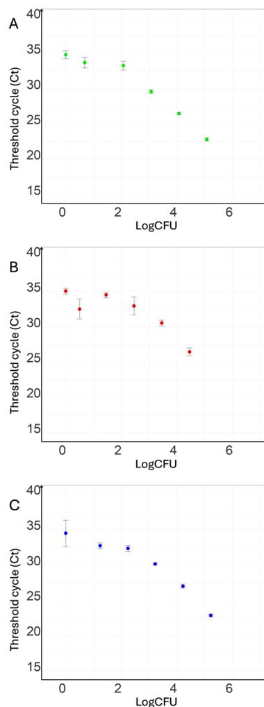
**Fig. 6** Bacteria DNA detection extracted in microfluidic siphons using qPCR. Real-time qPCR for *E. coli* detection in PBS (A) sheep blood (B) and river water (C). The plots show the median threshold cycle (Ct) values by CFUs of spiked *E. coli*  $\pm$  median absolute deviation of  $N = 3$  biological replicates and  $n = 3$  technical replicates.
