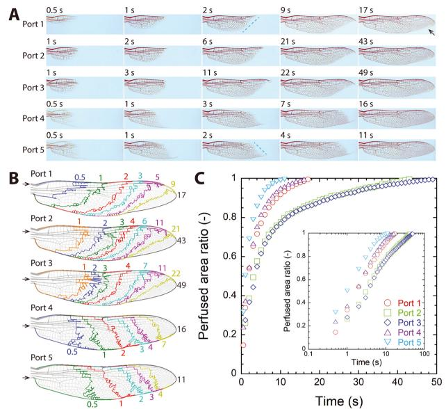
Fig. 3 Results of dye perfusion via single-port injection ( $Q = 5 \text{ mL min}^{-1}$ ). (A) Visualized perfusion of the injected dye. (B) Moving front of the dye through time. Colored numbers around each wing figure represent time in seconds, and the black number shown at the wing tip is the time to completely perfuse the device  $(t_{max})$ . Arrows indicate the port used for injection. (C) Temporal change of the perfused area ratio. Inset: log-linear plot.
