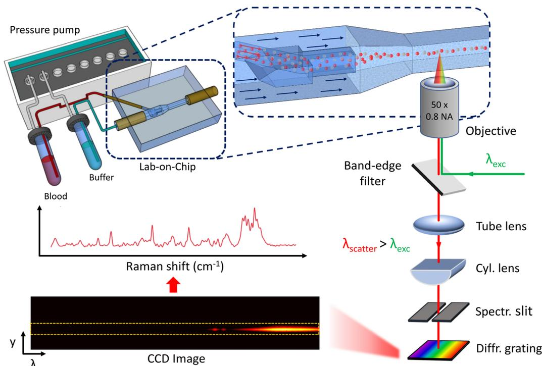
**Fig. 1** Schematic of the experimental setup. A pressure pump controls the focusing of the particles inside the Lab-on-a-Chip. The excitation light is focalized inside the chip via an objective, also used to collect the scattered light. This scattered light is reflected by a dichroic mirror and, after passing through a notch filter, is sent to the CCD camera inside a spectrometer, that enables us to extract the Raman spectra.
