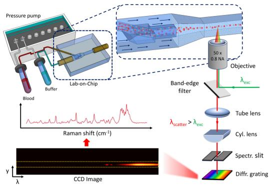
Fig. 1 Schematic of the experimental setup. A pressure pump controls the focusing of the particles inside the Lab-on-a-Chip. The excitation light is focalized inside the chip via an objective, also used to collect the scattered light. This scattered light is reflected by a dichroic mirror and, after passing through a notch filter, is sent to the CCD camera inside a spectrometer, that enables us to extract the Raman spectra.
