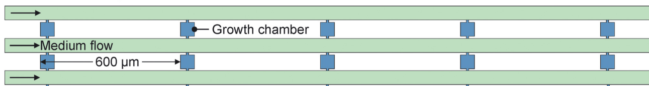
Fig. 2 Microfluidic cultivation chip layout. A: Cultivation chips of approximately 1 mm thickness (the cultivation layer) were used for experiments with CO 2 control to minimize the thickness of the gas exchange membrane. The second chip (the gas-control layer) was bonded onto the cultivation layer enabling the perfusion of air with defined CO 2 concentrations. B: Each chamber is connected to medium supply channels (10 μm height) resulting in a diffusive mass transfer within the chamber. The chambers have a surface area of 60 μm × 60 μm and a height of approximately 1 μm. C: The cultivation layer contains four 24 mm long arrays, each containing 8 rows of 40 evenly distributed growth chambers.
