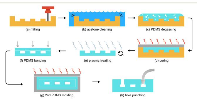
Fig. 12 Illustrated fabrication of PDMS microfluidic channels: (a) mill brass molds; (b) clean with sonication in acetone; (c) fill molds with uncured PDMS and degas; (d) cover and cure PDMS at 70 °C for 3 hours; (e) plasma treat cured PDMS; (f) bond PDMS microchannel; (g) embed microchannel in large PDMS mold; (h) hole punch cured microchannel for tube assembly.
