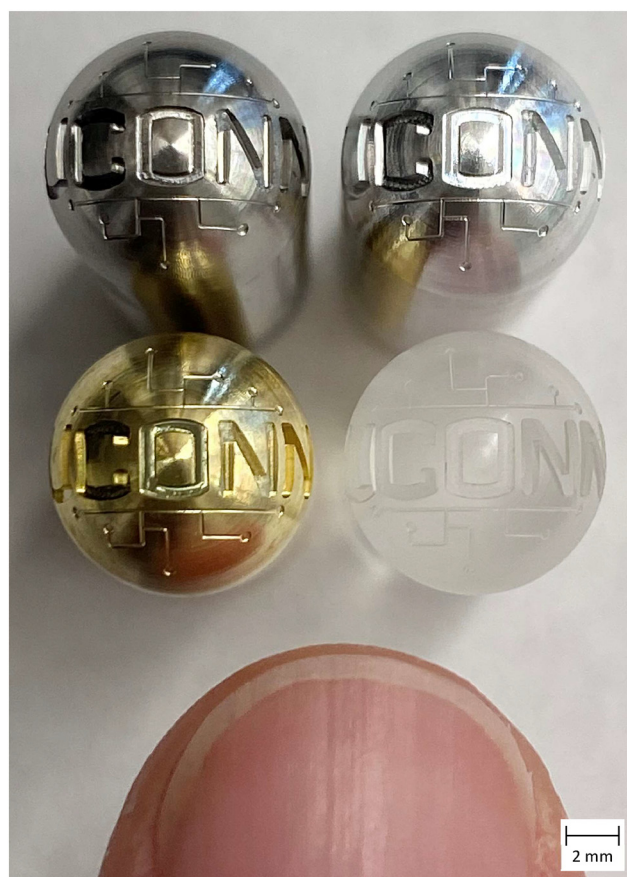
Fig. 7 Identical dome models milled from grade 5 titanium (top left), 360 brass (bottom left), 6061 aluminum (top right), and acrylic (bottom right) using the 5-axis CNC micro-milling machine, compared to human thumb nail.
