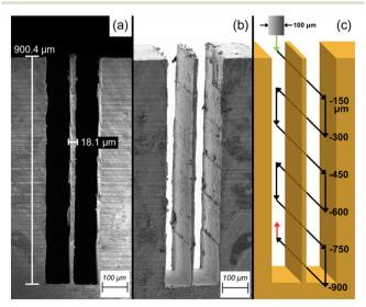
Fig. 4 SEM images of thin wall with 49.7:1 aspect ratio: (a) side view at 180× magnification; (b) angled view at 175× magnification; (c) illustration of toolpath.
