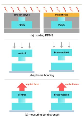
Fig. 10 Illustrated process for measuring the bond strength of plasma-bonded PDMS: (a) molding the surfaces of PDMS pillars from smooth acrylic and milled brass; (b) bonding the PDMS components using plasma treatment; (c) applying an increasing force until separation.
