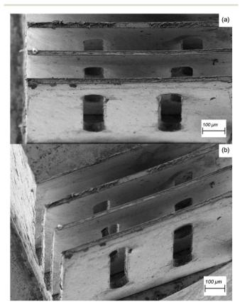
Fig. 6 SEM images of thin walls with side slots: (a) 250× magnification; (b) 200× magnification.
