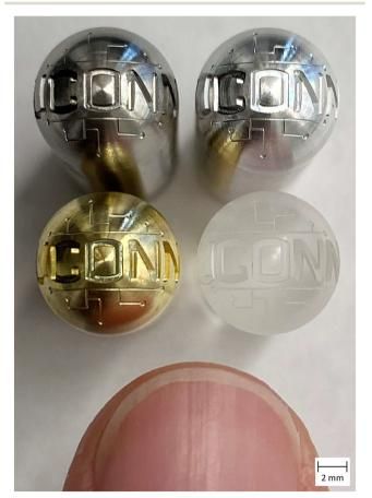
Fig. 7 Identical dome models milled from grade 5 titanium (top left), 360 brass (bottom left), 6061 aluminum (top right), and acrylic (bottom right) using the 5-axis CNC micro-milling machine, compared to human thumb nail.
