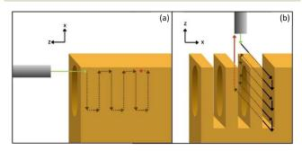
Fig. 5 Illustration of the milling toolpath for the thin walls with multiaxis milling features; (a) milling perpendicular slot; (b) milling thin
