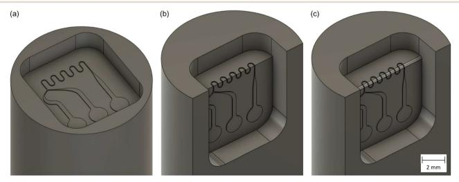
Fig. 11 CAD models of (a) channel 1 with a planar pattern, (b) channel 2 with a 90° edge, and (c) channel 3 with a rounded edge with a 250 μm radius of curvature.
