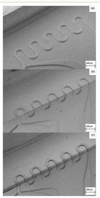
Fig. 15 SEM images of brass master molds at 45× magnification: (a) channel 1 (planar); (b) channel 2 (90 $^{\circ}$  edge); (c) channel 3 (250  $\mu m$ radius edge).
