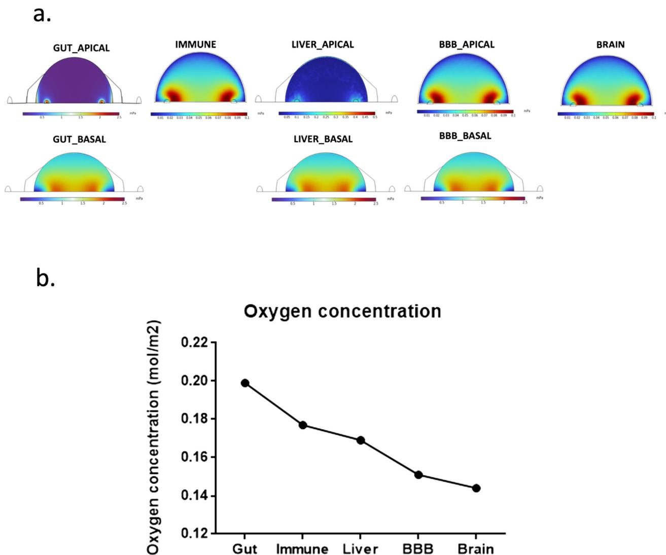
**Fig. 4** Computational fluid dynamics simulation of the PEGASO platform. (a) Shear stress (SS) on the upper side (top view) and lower side (bottom view) of the porous membrane separating the two culture chambers of the MINERVA 2.0 device. (b) Plot of the oxygen concentration profile through the OOCs of the PEGASO platform.
