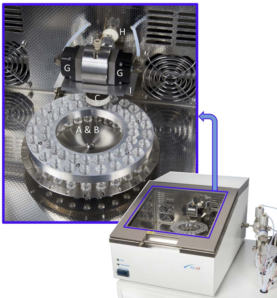
Fig. 2 Photograph of the inside of the Nu Sil sample chamber showing components illustrated in Fig. 1: the sample carousel with samples vials (A & B), the Nu Sil heater (C), the heat shield (I), vacuum valves (G), cleaning port (J) and outlet to the CF PREP cold finger (H). Other components shown in Fig. 1 are obscured in the view shown.
