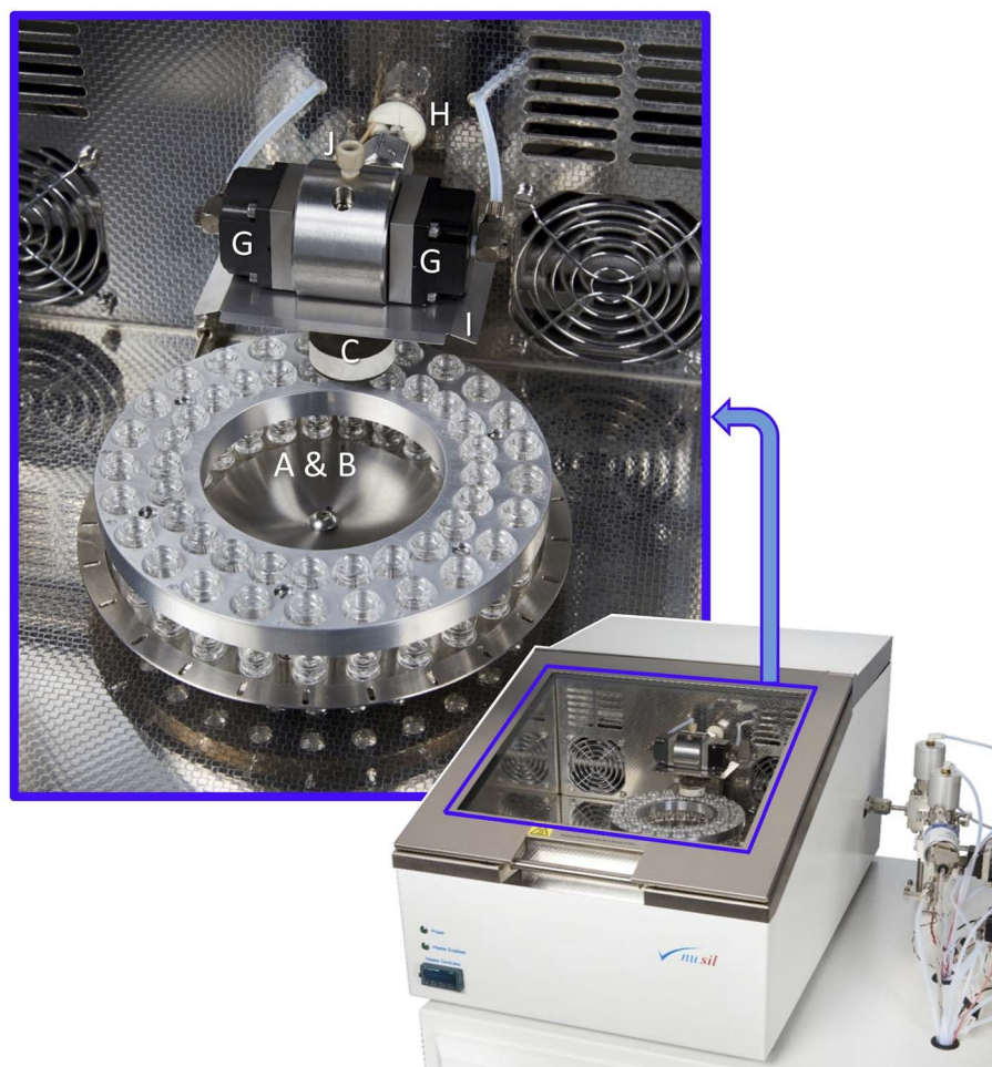
Fig. 2 Photograph of the inside of the Nu Sil sample chamber showing components illustrated in Fig. 1: the sample carousel with samples vials (A & B), the Nu Sil heater (C), the heat shield (I), vacuum valves (G), cleaning port (J) and outlet to the CF PREP cold finger (H). Other components shown in Fig. 1 are obscured in the view shown.
