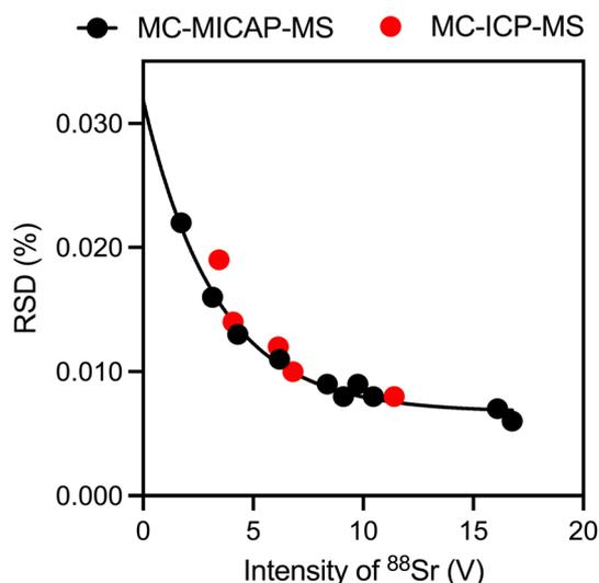
Fig. 3 Comparison of <sup>87</sup>Sr/<sup>86</sup>Sr intensity ratio precision, expressed as RSD (%), between MC-MICAP-MS and MC-ICP-MS (Ar-Neptune). Data collection: 75 runs at an integration time of 4.2 s.
