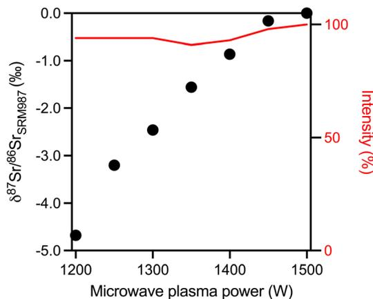
Fig. 6  $\delta^{87}\text{Sr}/^{86}\text{Sr}_{\text{SRM987}}$  and  $^{88}\text{Sr}^+$  intensity as a function of plasma power relative to the optimum power of 1500 W. Measurement precision (1 SD) is about 0.14‰ for the  $\delta^{87}\text{Sr}/^{86}\text{Sr}_{\text{SRM987}}$  values and ranges from 1.5% to 2.5% for the  $^{88}\text{Sr}^+$  intensities (see Fig. S3). For improved readability, no error bars are shown in the figure.
