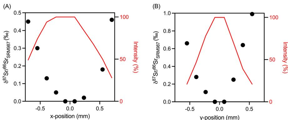
Fig. 4  $\delta^{87}\text{Sr}/^{86}\text{Sr}_{\text{SRM987}}$  and  $^{88}\text{Sr}^+$  intensity as a function of (A) x-position and (B) y-position of the torch relative to the optimum position (defined as 0 mm). Measurement precision (1 SD) ranges from 0.10‰ to 0.25‰ for the  $\delta^{87}\text{Sr}/^{86}\text{Sr}_{\text{SRM987}}$  values and from 0.5% to 5.0% for the  $^{88}\text{Sr}^+$  intensities (see Fig. S1). For improved readability, no error bars are shown in the figures.
