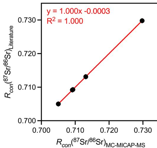
**Fig. 8** Correlation between conventional  $^{87}\text{Sr}/^{86}\text{Sr}$  isotope abundance ratios of geological and biological reference materials measured by MC-MICAP-MS and their reported conventional values in the literature (see Table 3). The error bars are smaller than the data points shown in the figure.
