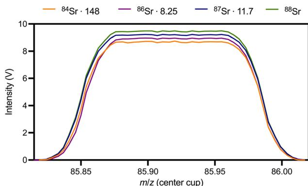
Fig. 2 Mass scan of 300 ng mL<sup>-1</sup> NIST SRM 987 solution in low resolution mode. Sample introduction using APEX Q (wet plasma).
