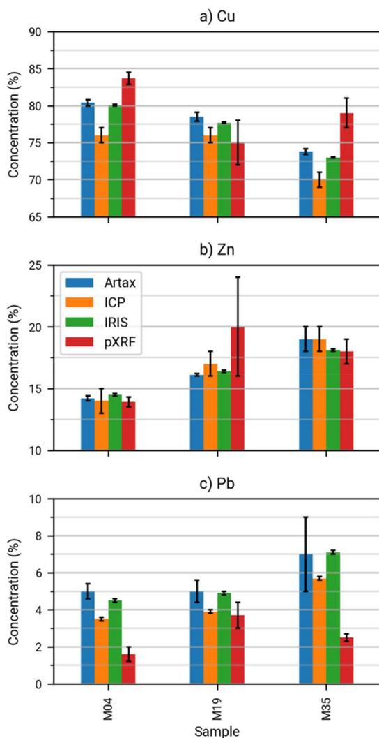
**Fig. 5** Comparison between the obtained data and the published data of (a) copper, (b) zinc, and (c) lead.<sup>5,18</sup>
