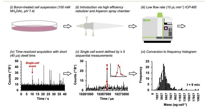
Fig. 3 Schematic single-cell ICP-MS (scICP-MS) workflow: (i) boron-treated cell suspension (100 mM ammonium acetate, pH 7.4); (ii) sample introduction *via* high efficiency nebulizer and Asperon spray chamber; (iii) low flow rate (10  $\mu$ L min<sup>-1</sup>) ICP-MS analysis; (iv) time-resolved acquisition with short (40  $\mu$ s) dwell time; (v) single cell event defined by ≥5 sequential measurements, (vi) conversion to frequency histogram.
