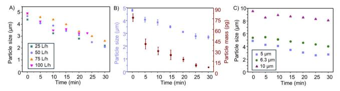
Fig. 2 (A) Optimisation of ozone flow rates using a 5  $\mu$ m PS standard, (B) assessment of degradation efficiency and method reproducibility based on particle size and mass using a 5  $\mu$ m PS standard (n=3), (C) evaluation of ozone's effect on particle size across 5, 6.3 and 10  $\mu$ m PS particles.
