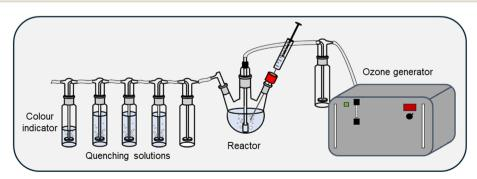
Fig. 1 Experimental setup for the degradation of microplastics using ozone.
