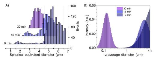
Fig. 3 Size distribution histograms of a 5  $\mu$ m PS standard after exposure to ozone for 0, 15 and 30 min, obtained by (A) SP ICP-MS and (B) DLS intensity distribution analysis.
