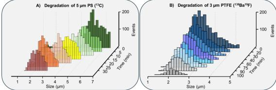
Fig. 4 Influence of ozone degradation on different polymer types. Calibrated size histograms of detectable MPs from: (A) a 5 µm PS standard targeting <sup>13</sup>C signal, and (B) a 3 µm PTFE standard targeting <sup>138</sup>Ba<sup>19</sup>F signal.
