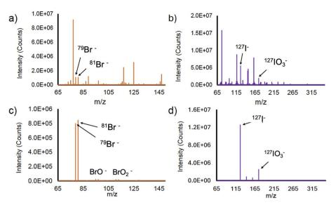
Fig. 2 Mass spectra derived from  $20 \,\mu\text{L}$  injections of  $10 \,\mu\text{g}$  mL $^{-1}$  halogen solutions illustrating the use of collisional dissociation. (a) NaBr, no CID, no HCD, (b) Nal, no CID, no HCD, (c) NaBr, CID = 40 eV, HCD = 20 eV and (d) Nal, CID = 40 eV, HCD = 20 eV. Discharge conditions: current = 60 mA, solution flow rate =  $60 \mu L min^{-1}$ , gas flow rate =  $600 mL min^{-1}$
