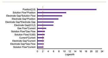
Fig. 4 Pareto plot representing bromide and iodide intensity responses across plasma conditions contained in design of experiment procedure. High logworth values indicate low p values and exemplify highly significant effects on the plasma performance. All logworth values below 1.3 were removed for simplicity.
