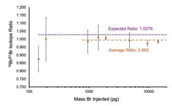
Fig. 6 Determined <sup>79</sup>Br/<sup>81</sup>Br isotope ratios obtained for triplicate 20 μL injections across a bromine mass of 0.019 to 191.2 ng, with the accepted isotope ratio and the value determined from the concentrations above the determined LOQ presented.
