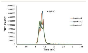
Fig. 5 Transient signals acquired from triplicate 20 μL injections of 2 ng Br in the form of NaBr for isotope ratio determinations, yielding a precision of 1.6% RSD for the integrated areas.
