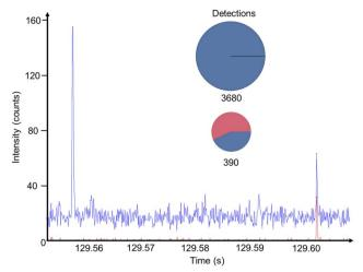
Fig. 5 Analysis of a mixture containing both aged PS and PVC MPs. PS and PVC were identified using an automated clustering, in which MP signals showing only a  $^{12}$ C<sup>+</sup> signal were identified as PS and MP events containing both  $^{12}$ C<sup>+</sup> and  $^{35}$ Cl $^{1}$ H $_{2}$ <sup>+</sup> signals were identified as PVC.
