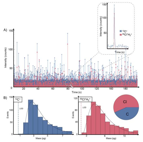
Fig. 4 (A) Transient raw data for the analysis of a PVC MP suspension. The signals  $^{12}$ C<sup>+</sup> and  $^{35}$ Cl<sup>1</sup>H<sub>2</sub> were monitored. A magnification for one selected SP event is provided on the top demonstrating the simultaneous detection of both Cl and C within the same particle. (B) shows mass distributions of detectable MPs containing both C and Cl and a pie chart showing the mass composition of the detected PVC particles.
