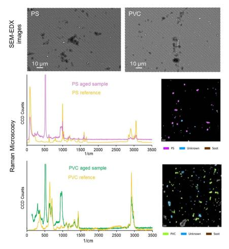
Fig. 1 Spectra and images recorded via SEM-EDX (top) and Raman microspectroscopy (bottom) of aged MPs generated from bulk PS and PVC are shown. The very strong band at 520 cm<sup>-1</sup> and broad band around 940 cm<sup>-1</sup> are attributed to the signals of the Si-filter.
