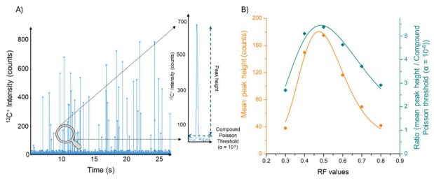
Fig. 2 Influence of RF values on  $^{12}$ C<sup>+</sup>-based MP detection using a 4  $\mu$ m PS standard: (A) SP event detection, including a zoomed-in view of one individual SP event. (B) Impact of RF set values on  $^{12}$ C<sup>+</sup> SP signal and signal-to-noise ratios. The signal-to-noise ratio was taken as the SP signal over the compound Poisson detection threshold ( $\alpha=10^{-6}$ ).
