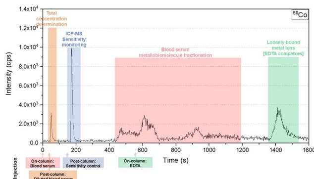
Fig. 1 SEC-ICP-MS chromatogram for <sup>59</sup>Co obtained from the analysis of Seronorm-L2, using the developed approach. The on-column or post-column injection time of blood serum (red), 8 mM EDTA (green), diluted blood serum sample (brown), and sensitivity control (blue) are indicated with an arrow below the x-axis. Peaks are assigned to the corresponding solution and indicated using their corresponding colour.
