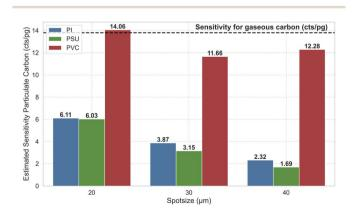
Fig. 6 Estimated sensitivity of particulate carbon for PI, PSU and PVC for the three spot sizes 20, 30, and 40  $\mu$ m in cts per pg. Additionally, the sensitivity for gaseous carbon is shown as a dashed line at 13.8 cts per pg.
