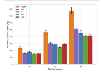
Fig. 3 Ablated carbon masses for the different spot sizes and polymer types investigated.
