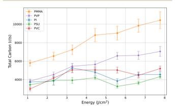
Fig. 1 Total carbon signal for the investigated polymers for different laser energies with a spot size of 30  $\mu$ m (n = 101 shots).
