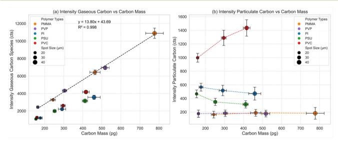
Fig. 4 Intensity of the gaseous carbon species vs. carbon mass (a) and intensity of particulate carbon vs. carbon mass (b). Calibration for gaseous carbon obtained by calculating a linear regression for the data of PMMA and PVP. Different amounts of carbon were introduced into the ICP-MS by ablating each polymer type with different spot sizes (20, 30, and 40 µm).
