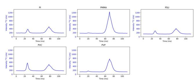
Fig. 2 Averaged SPRs for the 5 polymer types upon ablation with a 30  $\mu$ m spot size and 5.8 J cm<sup>-2</sup> laser energy. The first peak corresponds to particulate carbon species, whereas the second peak corresponds to gaseous carbon species. The start of the time axis is arbitrarily set to 0.
