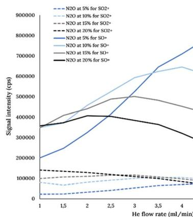
Fig. 5 The reaction efficiency under different He and N<sub>2</sub>O gas flow rates as signal intensities of <sup>32</sup>S<sup>16</sup>O and <sup>32</sup>S<sup>16</sup>O<sub>2</sub> product ions.
