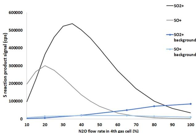
Fig. 4 The reaction efficiency and background signals under different flow rates of N<sub>2</sub>O gas as signal intensities of <sup>32</sup>S<sup>16</sup>O and <sup>32</sup>S<sup>16</sup>O<sub>2</sub> product ions.
