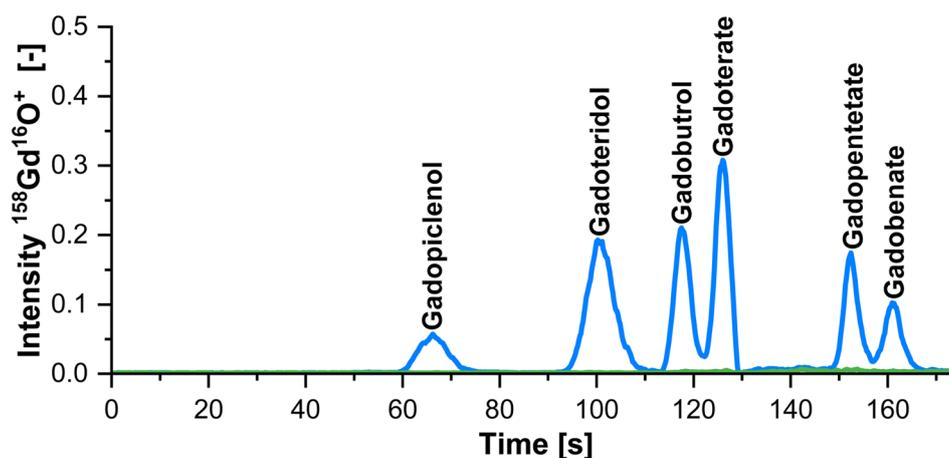
Fig. 2 IC-ICP-MS chromatogram of a 100 pM GBCA mix (blue) and a blank injection (green).  $^{158}\text{Gd}^{16}\text{O}^+$  intensity is normalised with the PCIS signal. GBCAs are labelled.
