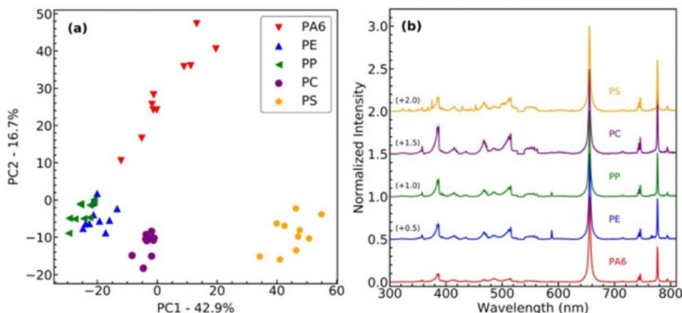
Fig. 1 Plastic type identification for PS, PC, PA6, PE, and PP. (a) shows a PCA with the first two principal components separating the plastic types into four clusters. (b) shows the reference average MPs spectra. Reproduced from ref. 12 with permission from Elsevier copyright [2025].
