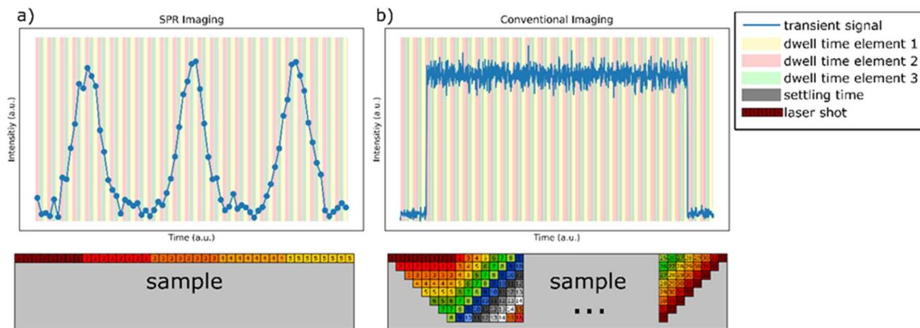
Fig. 2 Difference in the two measurement modes used for LA-ICP-MS imaging: (a) single-pulse response (SPR) imaging and (b) conventional imaging of a homogeneous distribution of an analyte.
