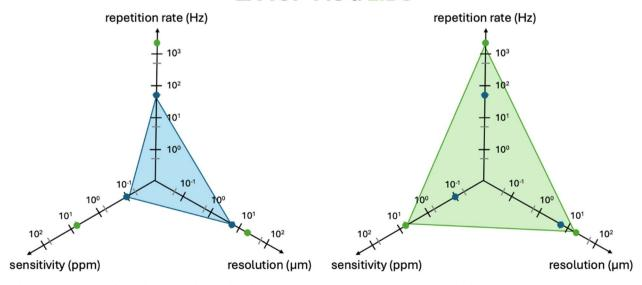
Fig. 5 Comparison of LIBS (green) and LA-ICP-MS (blue) parameters in terms of speed of analysis (Hz), sensitivity (ppm) and spatial resolution (μm).
