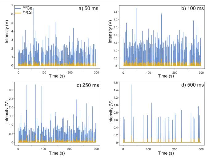
Fig. 2 Time traces for the cerium dioxide particles measured using (a) 50 ms, (b) 100 ms, (c) 250 ms, and (d) 500 ms integration times for the Faraday cup detectors. Only <sup>140</sup>Ce and <sup>142</sup>Ce are shown. As the integration time increases, the average intensity per particle decreases, and less particles are detected.
