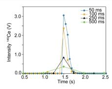
Fig. 3 One representative particle from each integration time is overlayed. Increasing the time of data collection on the Faraday cup (to 500 ms) decreases sensitivity (per particle). Shorter integration times tend to show a pattern of exponential decay after the initial 'spike', which is caused by detector decay from the particle signal input.
