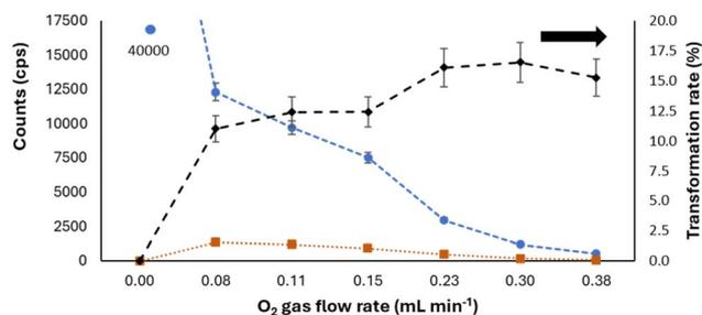
Fig. 1 Effect of the oxygen flow rate on the ionic signal obtained at *m/z* = 75 (blue circles), *m/z* = 91 (orange squares), and on the transformation rate (black circles, secondary axis). ICP-MS/MS operating conditions described in Table 1. As concentration: 25 μg kg<sup>-1</sup> using Conostan based solution.
