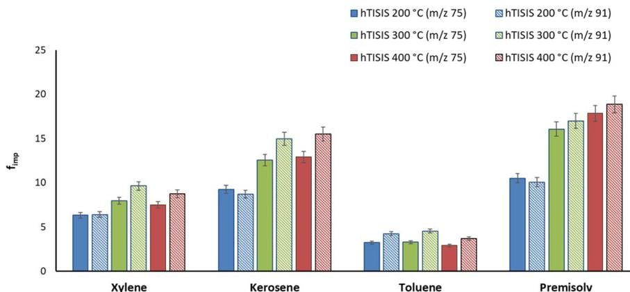
Fig. 2 Improvement factor ( $f_{\text{imp}}$ ) resulting from the use of hTISIS compared to a conventional sample introduction system for the four matrices evaluated and three hTISIS temperatures.  $Q_1^{\text{hTISIS}} = 30 \mu\text{L min}^{-1}$ ;  $Q_1^{\text{Conventional}} = 100 \mu\text{L min}^{-1}$ . ICP-MS/MS operating conditions described in Table 1. Oxygen gas flow rate to the reaction cell:  $0.075 \text{ mL min}^{-1}$ . As concentration using Conostan:  $25 \mu\text{g kg}^{-1}$ .
