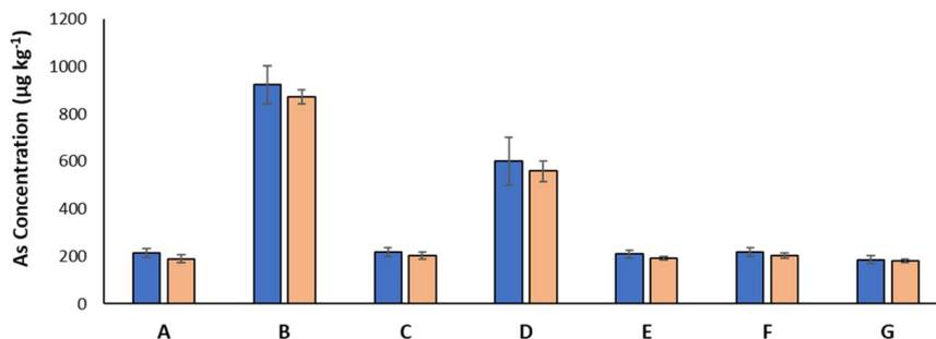
Fig. 4 Arsenic concentration ( $\mu\text{g kg}^{-1}$ ) for seven pyrolysis oil samples analyzed using the hTISIS at 400 °C. Calibration curve was prepared by using Conostan (blue bars) or TPA (orange bars).
