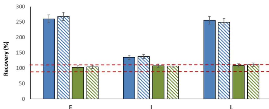
Fig. 5 Recoveries for a set of three TPO samples. Sample introduction system: Conventional (blue bars) and hTISIS at 400 °C (green bars). Solid-filled bars:  $m/z$  75 (on mass in MS/MS mode); and, hatched bars:  $m/z$  91 (mass-shift in MS/MS mode).
