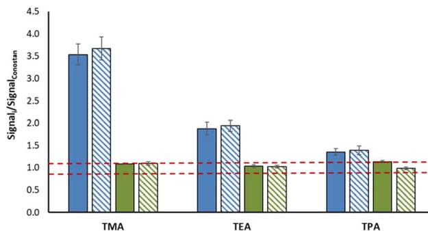
**Fig. 3** Relative signal found (mean value  $\pm$  standard deviation) for  $^{75}\text{As}^+$  and  $^{75}\text{As}^{16}\text{O}^+$  for different arsenic solutions, present under different chemical forms, using the conventional sample introduction system and the hTISIS at 400 °C. Sample introduction system: Conventional (blue bars) and hTISIS at 400 °C (green bars). Solid-filled bars:  $m/z$  75; and hatched bars:  $m/z$  91.
