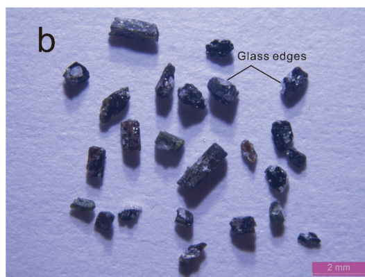
Fig. 4 Schematic diagram of the pretreatment equipment for the hornblende particles (a) and photographs of hornblende samples before (b) and after pretreatment (c). (b) Sample 10h1110h before pretreatment; (c) sample 10h1110h after pretreatment.
