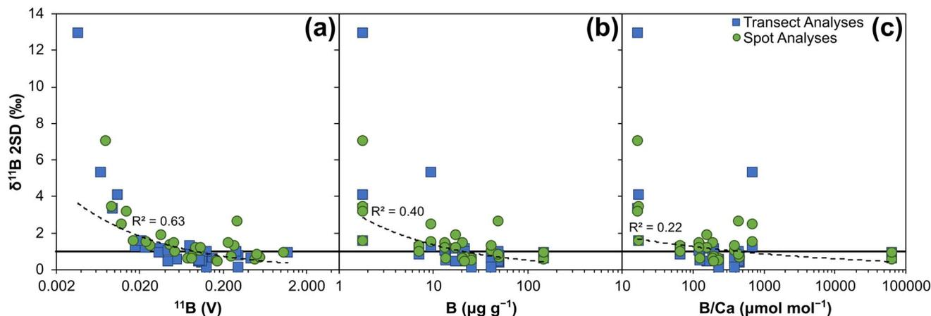
Fig. 5 Boron isotope external reproducibility (2SD) of 14 reference materials analysed by LA-MC-ICP-MS/MS: (a) plotted against  $^{11}\text{B}$  signal (V), (b) plotted against boron  $\mu\text{g g}^{-1}$ , and (c) plotted against B/Ca ( $\mu\text{mol mol}^{-1}$ ). Solid black line represents 2SD of 1‰. Dashed black line shows power relationship of all data, with  $R^2$  included.
