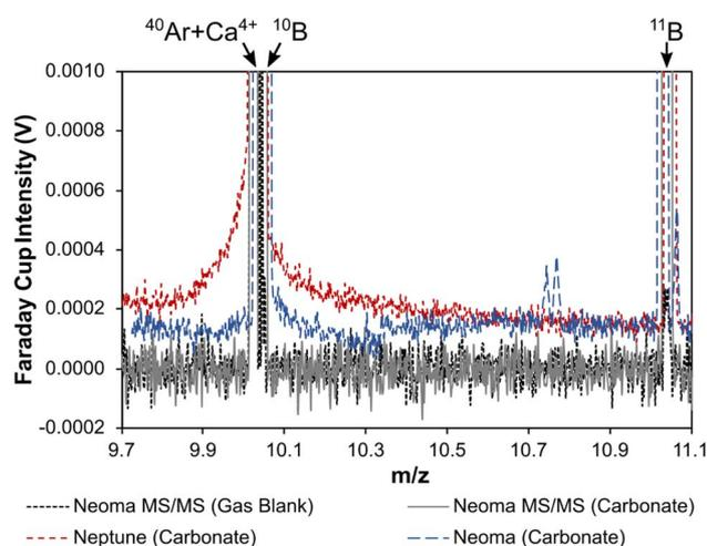
Fig. 6 Mass scans across the boron isotope mass range when ablating carbonate reference materials collected on a Neptune MC-ICP mass spectrometer,<sup>24</sup> Neoma MC-ICP mass spectrometer, and Neoma MS/MS MC-ICP mass spectrometer. A gas blank mass scan is also shown for the Neoma MS/MS MC-ICP mass spectrometer. Data from the scans are provided in ESI Table S6.†
