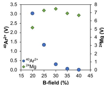
Fig. 8 Intensity of  $^{40}\text{Ar}^{2+}$  and  $^{24}\text{Mg}$  beams when a 100 ppb Mg solution is analysed on a Neoma MS/MS MC-ICP mass spectrometer with varying pre-cell mass filter  $B$ -fields. Data are available in ESI Table S7.†
