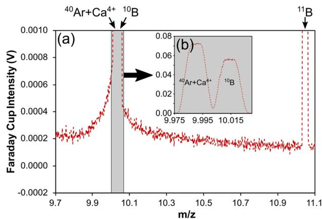
Fig. 1 (a) Mass scan across the boron isotope mass range when ablating a carbonate reference material collected on a Neptune MC-ICP mass spectrometer,<sup>24</sup> showing the elevated baseline across the entire boron mass range that acts as an interference and impacts the accuracy of boron isotope measurements by LA-MC-ICP-MS. (b) A mass scan showing the well-resolved  $^{40}\text{Ar} + \text{Ca}^{4+}$  and  $^{10}\text{B}$  peaks.
