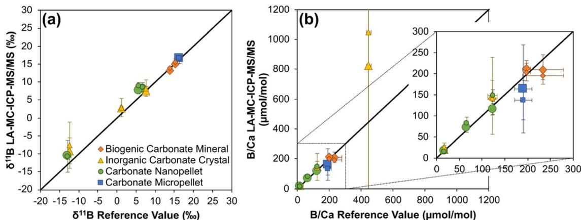
Fig. 10 Mean  $\delta^{11}\text{B}$  (a) and B/Ca (b)  $\pm 2$  SD for selected reference materials following normalisation to JCp-1. Solid black line represents 1 : 1 ratio. Data are available in ESI Tables S9 and S10.† Note that the large uncertainty on the inorganic carbonate crystals analysed is the result of small heterogeneity in B concentration of the target.
