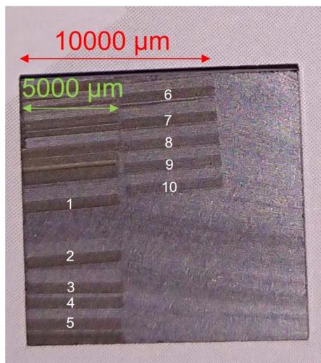
Fig. 1 Photograph of a WASO04 Si sample (natural isotopic composition) after laser ablation scans using  $\lambda = 213$  nm. The rectangular sample consists of a purified single crystal with approximately 15 mm  $\times$  15 mm. Lengths of ablation scan lines were approximately 5000  $\mu\text{m}$ . Numbers indicate the line scans and corresponding sequences used for isotope ratio measurements.
