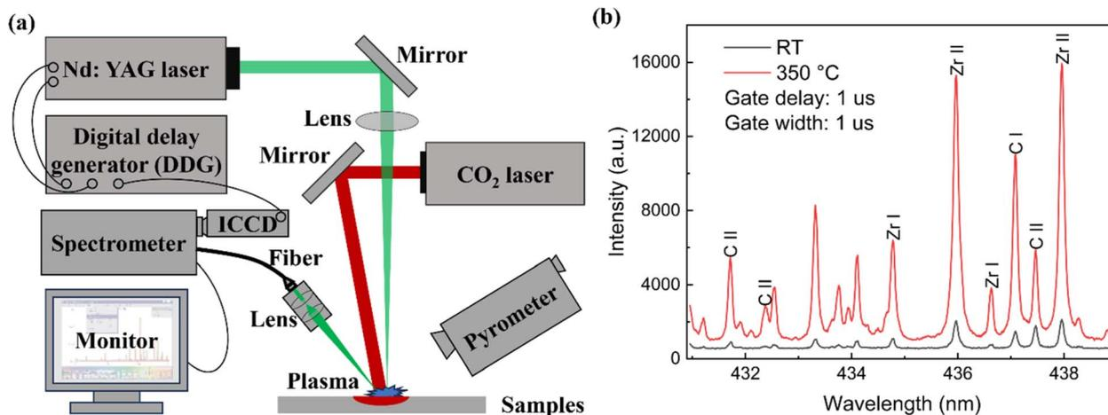
Fig. 1 (a) Schematic of the LIBS experimental setup and (b) typical LIBS spectra obtained from the ZrC surface at room temperature and 350 °C.
