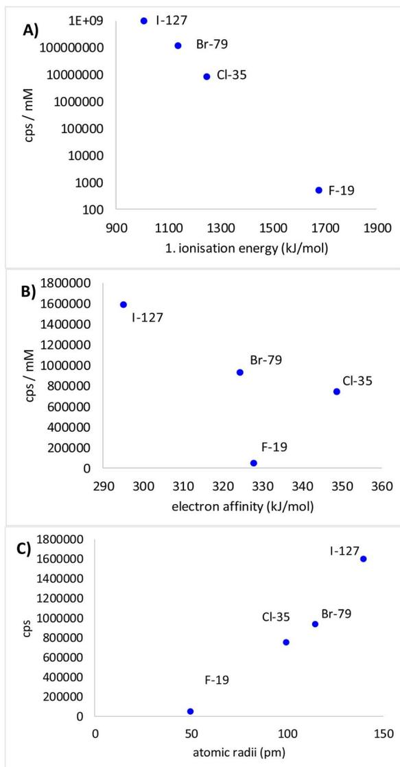
Fig. 5 Dependence of signal intensity on (A) ionization energy for medium resolution-nICPMS (data from Bu *et al.*<sup>24</sup>) and (B) (cps per mM isotope) electron affinity for nICPMS; (C) atomic radii for nICPMS and the dependence of signal intensity (cps per mM) on these parameters.
