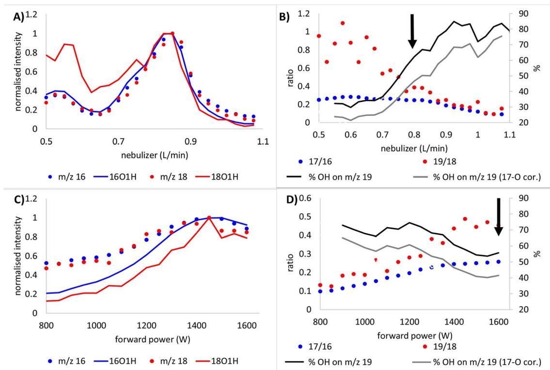
**Fig. 8** (A) and (C) The dependence of signal intensity (blank solution) vs. (A) nebulizer gas flow rate (at forward power 1600 W) and (C) vs. forward power (at nebulizer gas flow rate of 0.8 L min<sup>-1</sup>), panels (B) and (D) show the calculated ratios  $m/z$  17/16 and  $m/z$  19/18 plus the estimated relative contribution of OH to the signal at  $m/z$  19 (max–min); eqn (1–2d) used for calculations; black arrow indicates the area of highest sensitivity.
