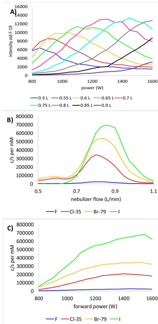
Fig. 4 A) An example of fluorine ( $m/z$  19) intensity variation with forward power at set nebulizer gas flow rates; (B) signal intensity (in cps per mM Hal) versus nebulizer gas flow rate at 1600 W (C) signal intensity (in cps per mM Hal) versus forward power for a nebulizer gas flow rate of 0.8 L Ar per min (sample  $10 \text{ mg L}^{-1}$  halogen mix).
