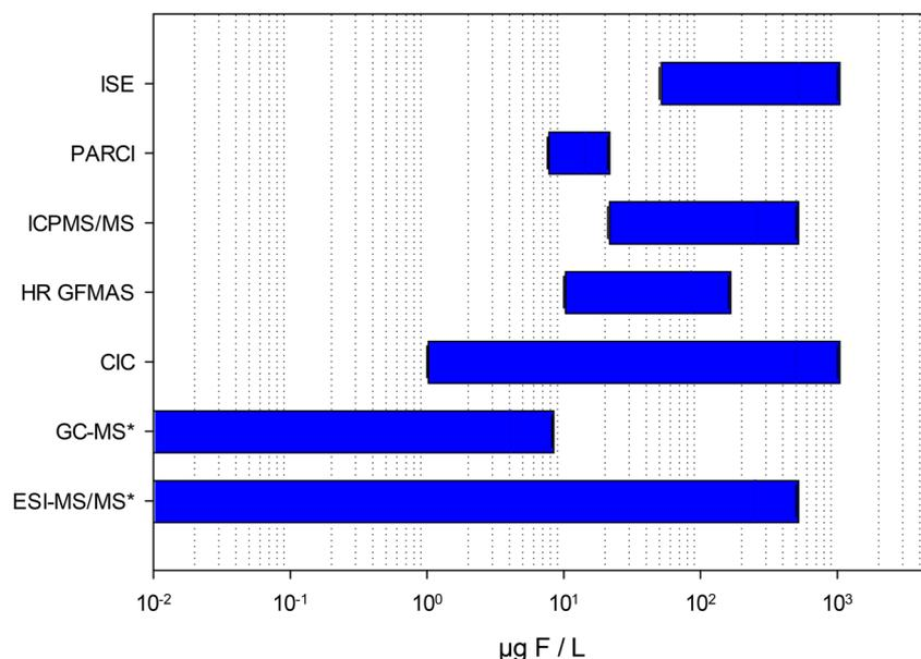
Fig. 1 Estimated instrumental detection limits for fluorine (\*: fluorinated compounds) taken from various literature sources; ESI-MS/MS, GC-MS and PARCI data from flow injection or in combination with a separation technique; for chlorine and bromine detection limits are similar except for ICPMS/MS where they are lower (est.  $0.01\text{--}0.1 \text{ } \mu\text{g L}^{-1}$ ). Table S2† shows some additional detection limits for F, Cl and Br from the literature.
