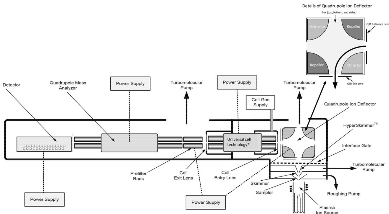
Fig. 2 Instrument set-up Nexion2000<sup>®</sup>.
