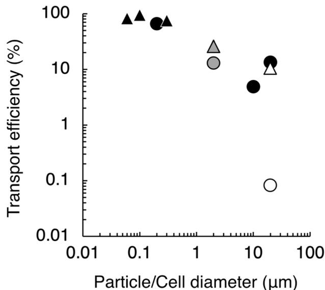
Fig. 2 Transport efficiencies of SiO<sub>2</sub>, Ag, and TiO<sub>2</sub> particles, yeast cells, and K562 cells. Black circle: SiO<sub>2</sub> particle, gray circle: yeast cell, white circle: K562 cell using the conventional sample introduction system for sICP-MS. Black triangle: Ag and TiO<sub>2</sub> nanoparticle, gray triangle: yeast cell, white triangle: K562 cell using μDG-ICP-MS. Data represent the average values of three repeated measurements. Error bars (SD) are included in each symbol.
