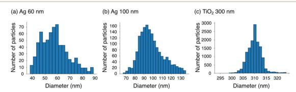
Size distributions of nanoparticles obtained by  $\mu$ DG-ICP-MS. (a) Ag 60 nm, (b) Ag 100 nm, and (c) TiO<sub>2</sub> 300 nm.
