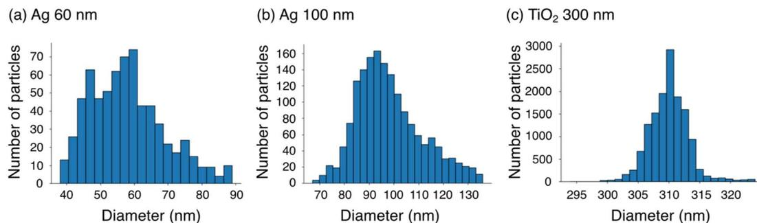
Fig. 5 Size distributions of nanoparticles obtained by  $\mu$ DG-ICP-MS. (a) Ag 60 nm, (b) Ag 100 nm, and (c) TiO<sub>2</sub> 300 nm.
