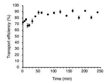
Fig. 7 Transport efficiency of  ${\rm TiO_2}$  nanoparticles introduced by using  ${\rm \mu DG}$  over 4 h.
