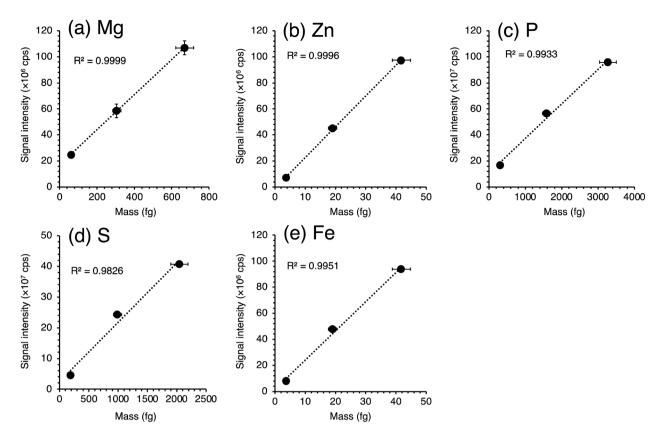
Fig. 4 Calibration curves of five essential elements obtained from microdroplets of ionic standard solutions for K562. (a) Mg, (b) Zn, (c) P, (d) S, and (e) Fe.
