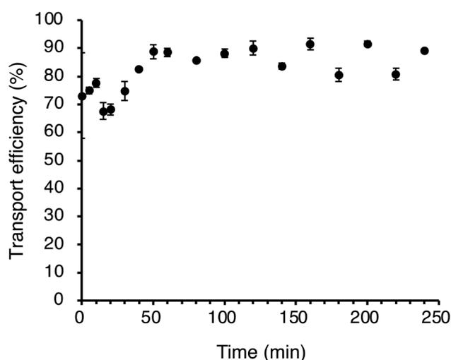
Fig. 7 Transport efficiency of TiO<sub>2</sub> nanoparticles introduced by using  $\mu$ DG over 4 h.
