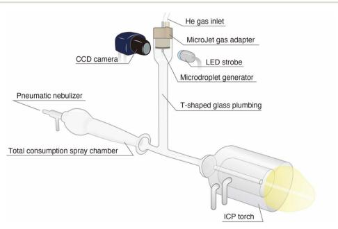
Fig. 1 Configuration of the sample introduction system with μDG.
