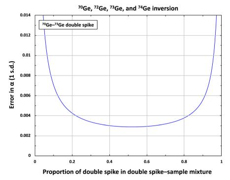
Fig. 2 Propagation of the theoretical uncertainties (error) on the natural fractionation coefficient  $\alpha$  as a function of the proportion of Ge double spike in the spike–sample mixture calculated using the Double Spike Toolbox and using  $^{70}$ Ge,  $^{72}$ Ge, and  $^{74}$ Ge for the inversion.  $^{29}$
