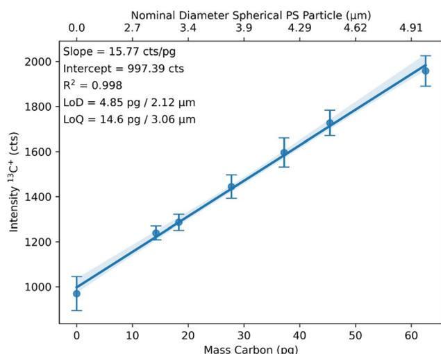
Fig. 3 Generated linear calibration function showing the relation between the intensity for the  $^{13}\text{C}^+$  signal and the mass of carbon (lower  $x$ -axis) and, respectively, the nominal diameter of a spherical PS particle (upper  $x$ -axis).
