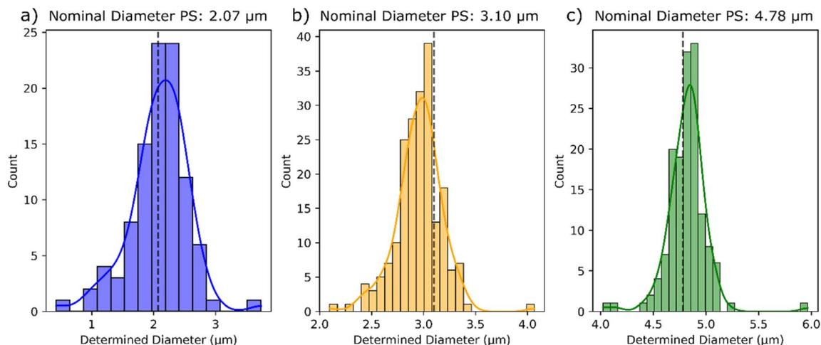
Fig. 4 Size distribution of the evaluated PS microplastic particles for the 2.07  $\mu\text{m}$  particles (a), the 3.10  $\mu\text{m}$  particles (b), and the 4.78  $\mu\text{m}$  particles (c), including a Kernel density estimation curve and the nominal certified diameters marked with the dotted black lines.
