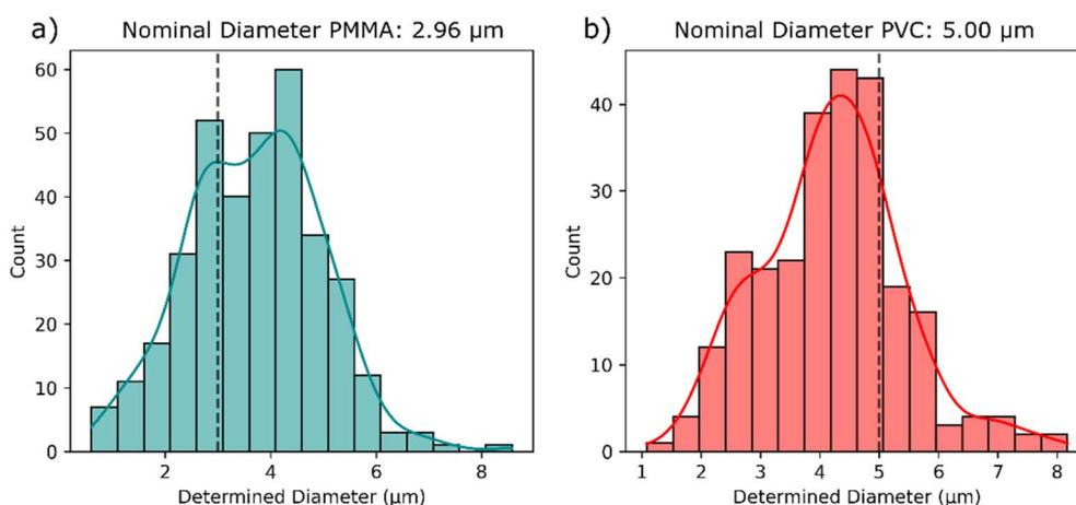
Fig. 5 Size distribution of the evaluated microplastic particles for the 2.96  $\mu\text{m}$  PMMA particles (a) and the 5  $\mu\text{m}$  PVC particles (b), including a Kernel density estimation curve and the nominal certified diameters marked with the dotted black lines.
