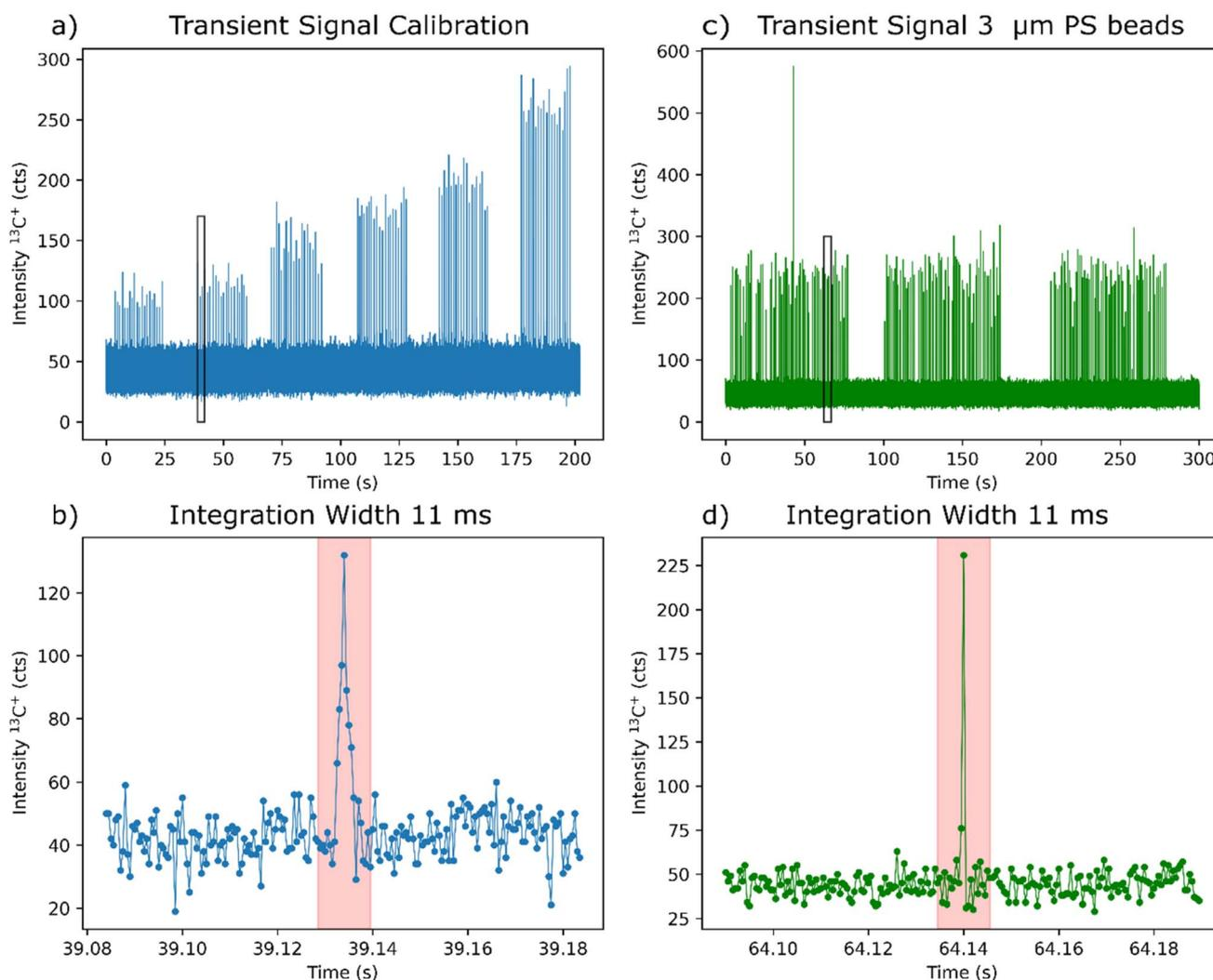
Fig. 2 Transient signals for  $^{13}\text{C}^+$  using a laser fluence of  $1.4 \text{ J cm}^{-2}$ , dwell time of  $500 \mu\text{s}$  and a KED gas flow of  $0.6 \text{ mL min}^{-1}$  for the calibration standards (a) and the for the  $3 \mu\text{m}$  PS particles exemplarily (c) with corresponding zoomed figures (b) and (d) showing the black framed rectangles in the top figures enlarged.
