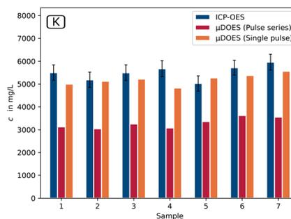
Fig. 7 Comparison of the micro-discharge OES potassium results with laboratory ICP-OES data based on selected samples of the ore leaching process step (on-line  $\mu$ DOES:  $n = 1$  continuous process and ICP-OES:  $n = 5$ ).
