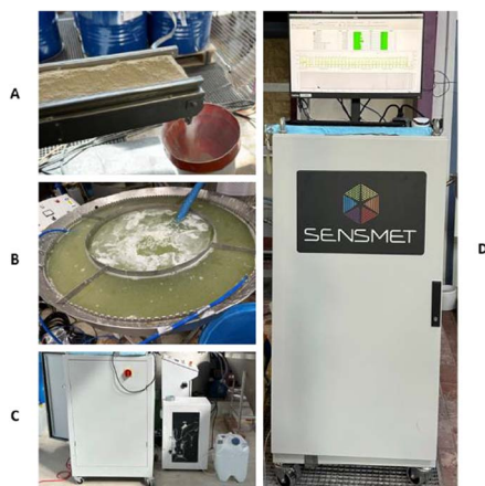
Fig. 2 On-site setup and sampling point exemplary for the first process step (A: addition of the calcined lithium ore, B: clarifier with the product, C: analyser, dilution unit and ultrapure water supply, and D: analyser front view with operating software).
