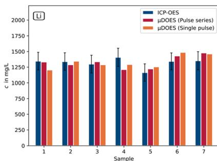
Fig. 5 Comparison of the micro-discharge OES lithium results with laboratory ICP-OES data based on selected samples of the ore leaching process step (on-line  $\mu\text{DOES}$ :  $n = 1$  continuous process and ICP-OES:  $n = 5$ ).
