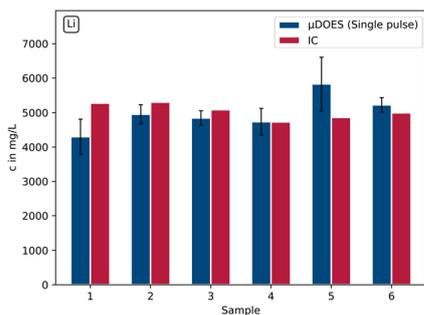
Fig. 8 Comparison of Li concentrations measured by micro-discharge OES and ion chromatography using selected samples of the lithium carbonate precipitation process step (batch-wise  $\mu$ DOES:  $n = 3$  and IC:  $n = 1$  due to long measurement time).
