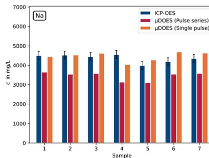
Fig. 6 Comparison of the micro-discharge OES sodium results with laboratory ICP-OES data based on selected samples of the ore leaching process (on-line  $\mu\text{DOES}$ :  $n = 1$  continuous process and ICP-OES:  $n = 5$ ).
