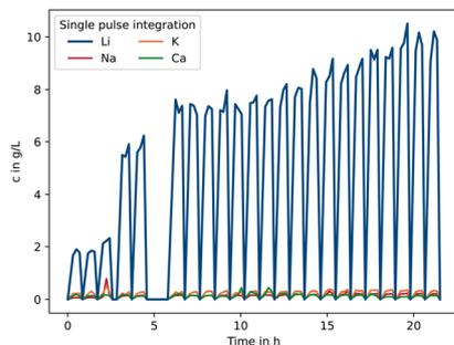
Fig. 9 Increase in lithium concentration with increasing process time and addition of lithium carbonate to the  $\text{Ca}(\text{OH})_2$  suspension.
