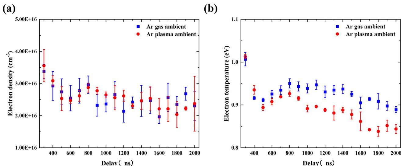
Fig. 5 Temporal evolution of space-integrated (a) electron density and (b) electron temperature of W plasma under Ar gas ambient and Ar plasma ambient.
