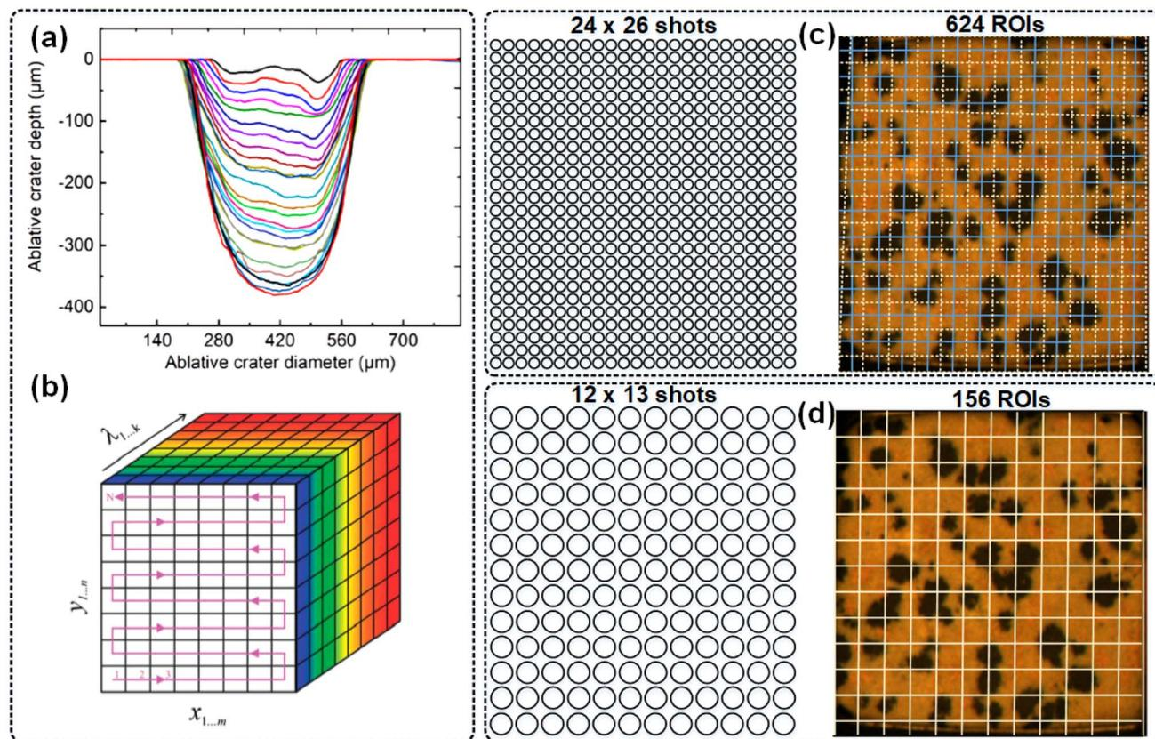
Fig. 2 LIBS imaging operation.<sup>25,30,31</sup>
