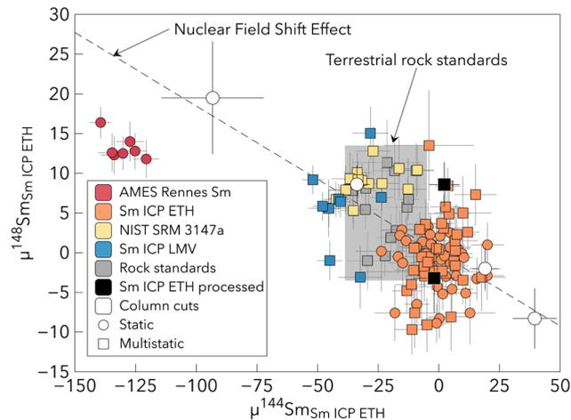
Fig. 7 Diagram comparing  $\mu^{144}\text{Sm}$  and  $\mu^{148}\text{Sm}$  compositions of all synthetic and terrestrial rock standards measured during this study, normalised to the Sm ICP ETH standard measured during the corresponding session. The column cuts (white circles) measured individually aligned along the NFSE trend. All standards, except AMES Rennes Sm were broadly aligned on this trend. Terrestrial rock standards plot next to the composition of NIST SRM 3147a.
