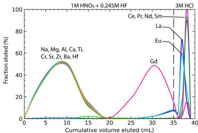
**Fig. 1** Elution curves for step 2 using TRU-Spec resin to separate LREE from matrix elements. A basalt (RU0701) from the Réunion Island in the Indian Ocean<sup>44</sup> was used for the calibration. Matrix elements and high-field strength elements were removed during the loading and rinsing steps in 1 M HNO<sub>3</sub>–0.245 M HF. Neodymium and samarium were stripped off the column using 3 M HCl. Most of the Gd and heavier REE were eluted in the first step of the procedure.
