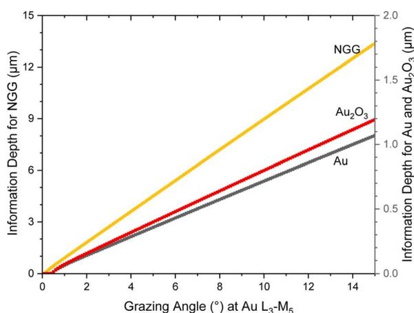
Fig. 3 Information depth at various exit angles for Au,  $Au_2O_3$ , and NGG at Au  $L_3$ - $M_5$  fluorescence line calculated from CXRO website<sup>36</sup> [last accessed 24.06.2024].
