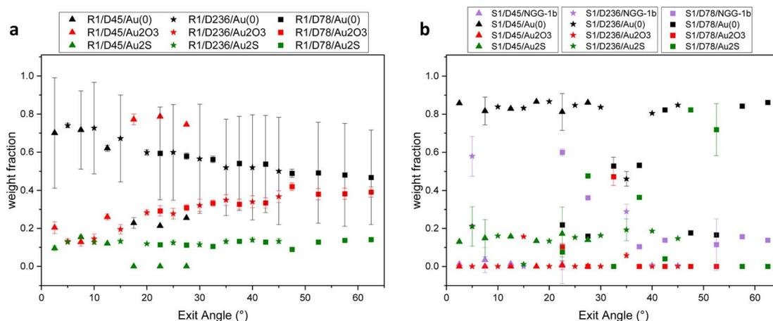
Fig. 5 Angular dependence of gold speciation as obtained from LCF of simultaneous Au  $L_{\alpha}$  AR-XANES from the three sets of detector arrays for (a) reference sample R1 and (b) replica sample S1. Black represents Au(0), red: Au<sub>2</sub>O<sub>3</sub>, green: Au<sub>2</sub>S, and purple represents Nanogold Gel NGG-1b.
