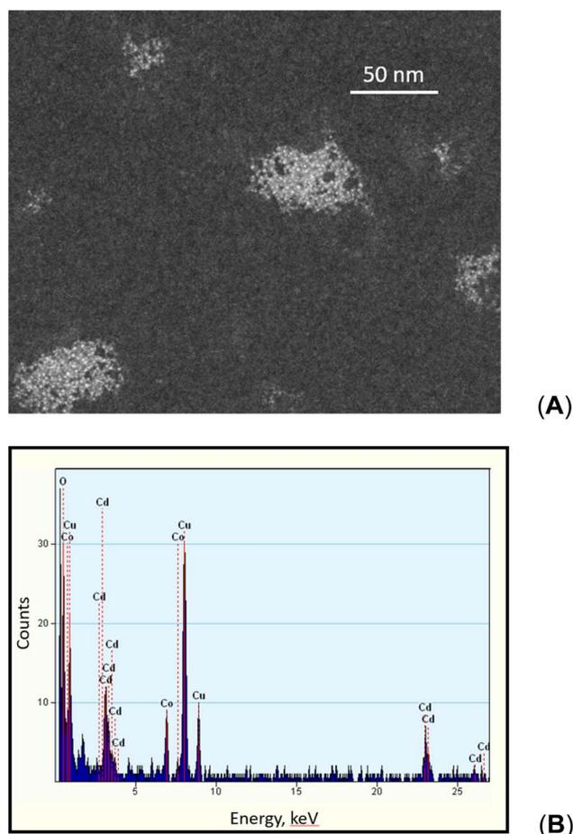
Fig. 16 (A) TEM image of clusters of mixed Cd/Co comprising NPs of diameter < 5 nm synthesized during PVG of 0.045% (v/v) formic acid containing 50 μg mL<sup>-1</sup> Cd(II)/100 μg mL<sup>-1</sup> Co(II); (B) EDX profile of a cluster (images courtesy of M. Couillard, EME/NRC).
