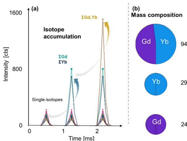
Fig. 3 (a) Shows one function of the in-built calculator. NPs containing Yb and Gd can be detected based on individual isotopes. However, isotopes for each element can be accumulated to increase signal to noise ratios and even signals from different elements can be summed up to improve figures of merit further. (b) Shows a HAC analysis of the analysed NP sample and determined 3 clusters with different element composition.
