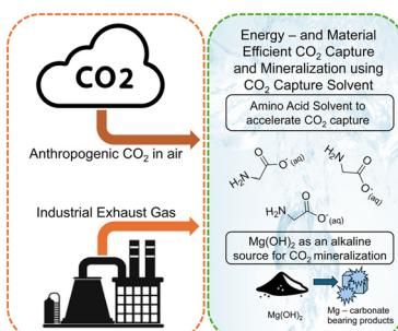
Reactive CO<sub>2</sub> capture and mineralization of magnesium hydroxide to produce hydromagnesite with inherent solvent regeneration
