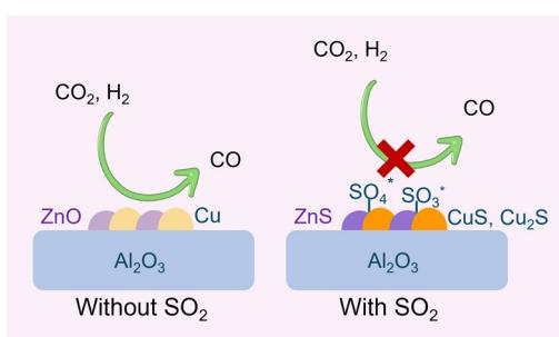
Deactivation mechanisms of Cu-Zn-Al<sub>2</sub>O<sub>3</sub> in CO<sub>2</sub> hydrogenation induced by SO<sub>2</sub> exposure
