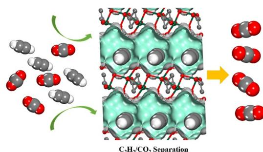
Scalable copper-based coordination frameworks with tailored pore chemistry for energy-efficient C<sub>2</sub>H<sub>2</sub>/CO<sub>2</sub> separation
