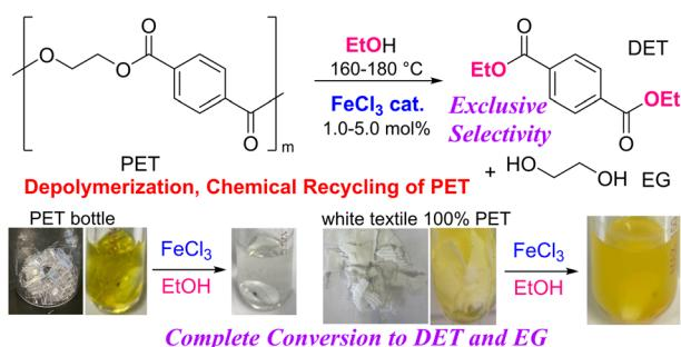
**Depolymerization of PET with ethanol by homogeneous iron catalysts applied for exclusive chemical recycling of cloth waste**
