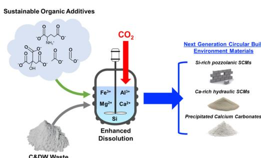
**Carboxylic ligands to enhance material recovery from construction waste to produce CaCO<sub>3</sub> for carbon utilization**
