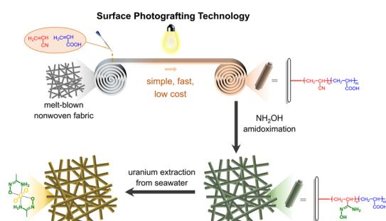
**Toward a low-cost uranium-adsorbing material based on nonwoven fabrics and photografting technology**
