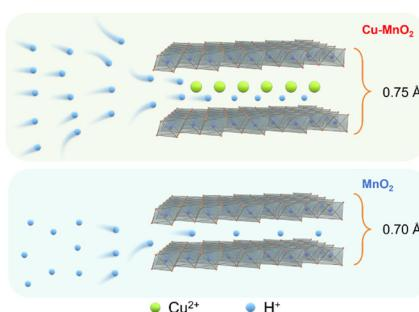
**Copper ions-intercalated manganese dioxide self-supporting mesoporous carbon electrode for aqueous zinc-ion batteries**
