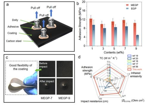
Fig. 7 Mechanical properties and literature comparison of the coatings (a and b) pull-off adhesion and (c) impact resistance test of the coatings. Comparisons of our MEGP-9 coating with some reported carbon-based high TC protective coatings in terms of TC, infrared emissivity, adhesion strength, impact resistance and  $|Z|_{0.01Hz}$  performances, where 0 indicates that the corresponding performance was not evaluated in the study (d).
