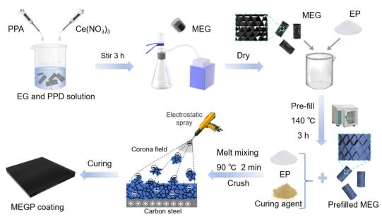
Fig. 1 Schematic of MEGP coating preparation. The composite coating MEGP was prepared through a melt pre-filled process, melt mixing and powder spraying.
