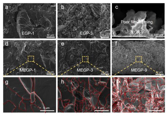
Fig. 3 Morphology of coatings: SEM section images of EGP (a-c) and MEGP (d-i) with different filler contents.
