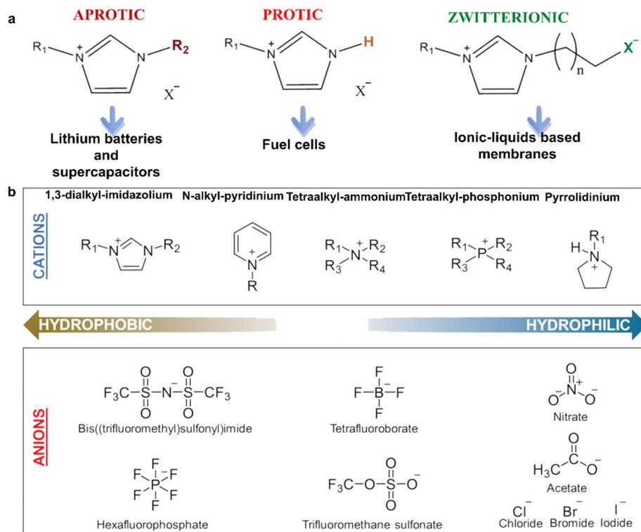
**Fig. 3** ILs classification and structure diagram. (a) General classification of ionic liquids with an indication of a representative application area;<sup>41</sup> (b) schematic representation of the most common cations and anions described in the literature. Reproduced with permission.<sup>44</sup> Copyright 2009, Springer Nature; 2013, RSC.
