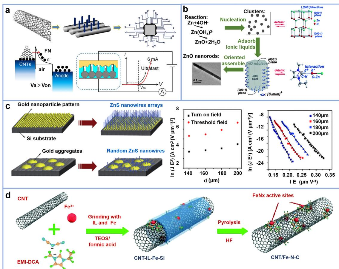
**Fig. 5** Representative roles of ILs in 1D EIMs. (a) CNT-based air-channel device;<sup>85</sup> (b) IL-induced growth of ZnO nanorods;<sup>93</sup> (c) IL-guided assembly of ZnS nanowires on gold templates;<sup>99</sup> (d) IL-assisted synthesis of CNT/Fe-N-C electrocatalysts for ORR.<sup>101</sup> Copyright 2023, ACS and 2011, 2021, RSC.
