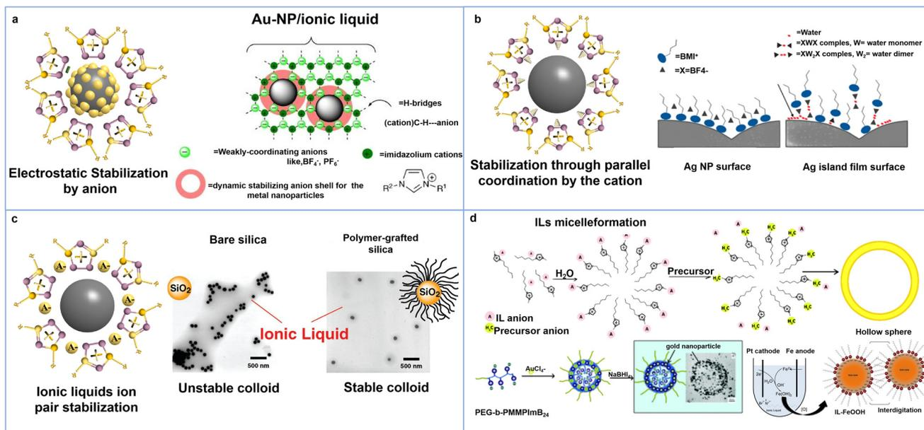
Fig. 4 ILs-guided 0D material construction: (a) anion-based electrostatic stabilization;<sup>45</sup> (b) cation coordination;<sup>74</sup> (c) ion-pair stabilization;<sup>75,76</sup> (d) micelle formation.<sup>45,77,78</sup> Copyright 2008, ACS; 2014, RSC and 2016, Elsevier.
