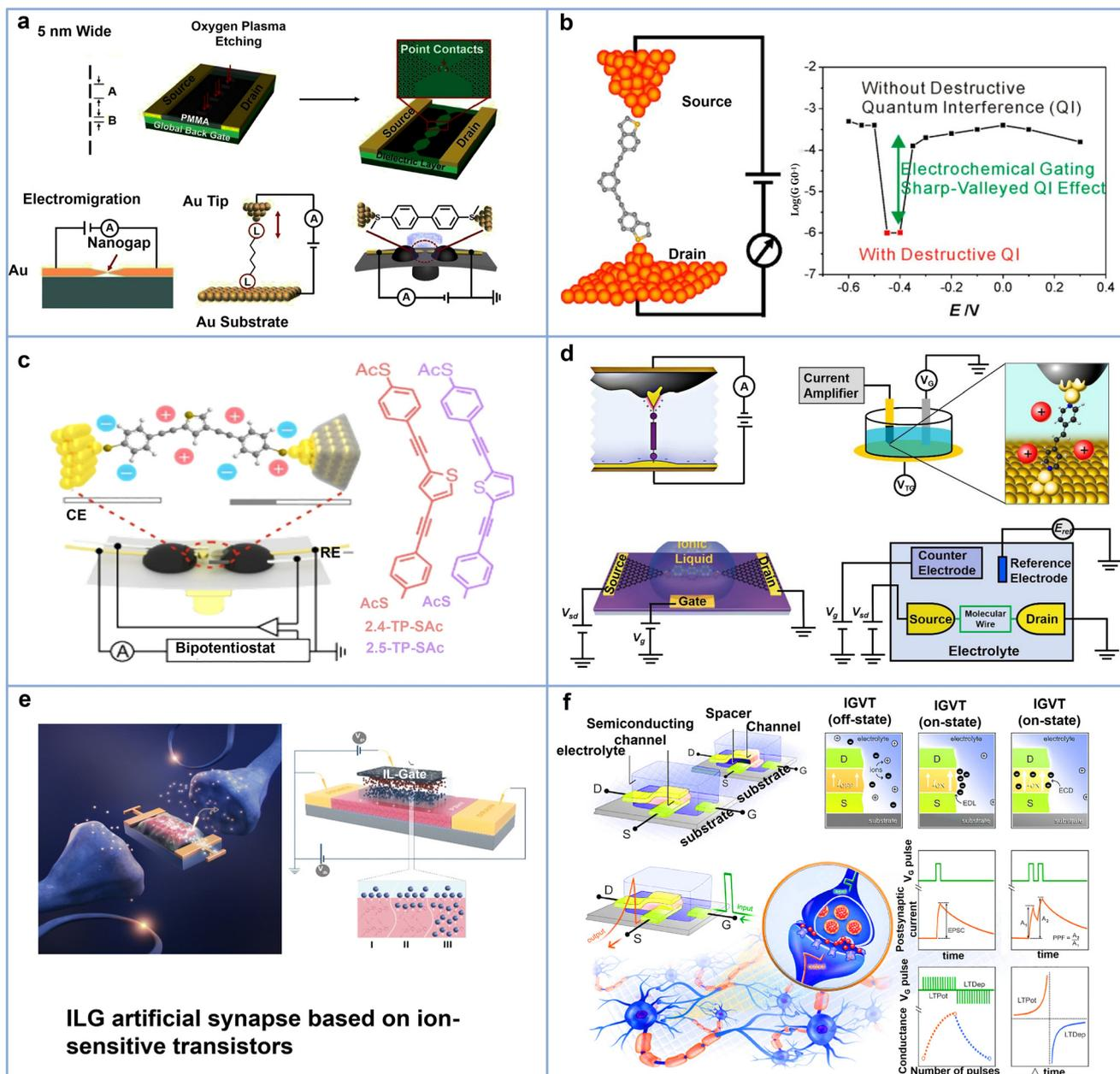
Fig. 8 IL-enabled electronic devices: (a) ILG single-molecule junctions;<sup>22</sup> (b) *para/meta*-BT conductance profiles;<sup>25</sup> (c) molecular structures of 2,5-/2,4-TP-SAC;<sup>26</sup> (d) IL-assisted single-molecule transport characterization;<sup>171</sup> (e) ILG artificial synapse based on ion-sensitive transistors;<sup>172</sup> (f) IL-gated neuromorphic array for synaptic modulation.<sup>173</sup> Copyright 2024, ELSEVIER; 2023, WILEY and 2019, Springer Nature.
