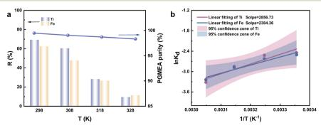
Fig. 7 (a) Effect of temperature on metal ion removal efficiency and purity of PGMEA after resin adsorption; (b) the curve of the thermodynamic model for metal ion adsorption onto resin.
