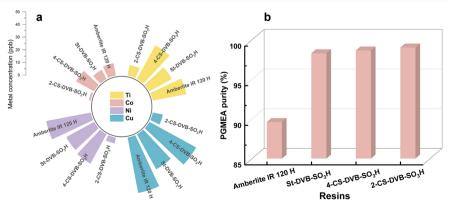
Fig. 1 (a) The concentration of metal ions in PGMEA after adsorption with different resins; (b) the purity of PGMEA after adsorption with different resins.
