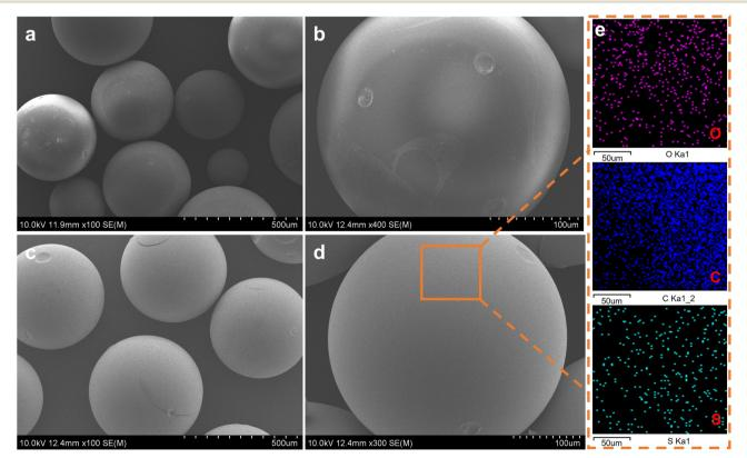
Fig. 2 (a) SEM image of gel polymers with a resolution of 500 μm; (b) SEM image of a gel polymer with a resolution of 100 μm; (c) SEM image of sulfonated gel polymers with a resolution of 500 μm; (d) SEM image of a sulfonated gel polymer with a resolution of 100 μm; (e) EDS mapping images of the sulfonated gel polymer.
