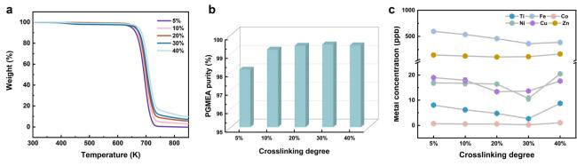
Fig. 3 (a) Thermogravimetric curves of gel polymers at different crosslinking degree; (b) the purity of PGMEA after adsorption with resins at different crosslinking degree; (c) the concentration of metal ions in PGMEA after adsorption with resins at different crosslinking degree.
