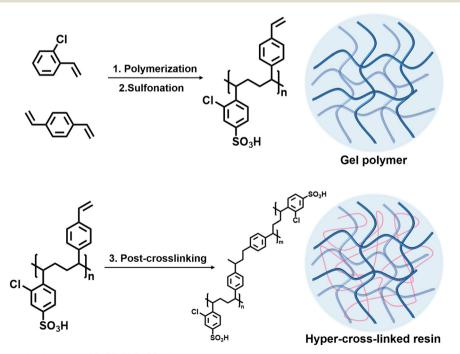
Scheme 1 The complete synthesis route of 2-CS-DVB-SO<sub>3</sub>H.
