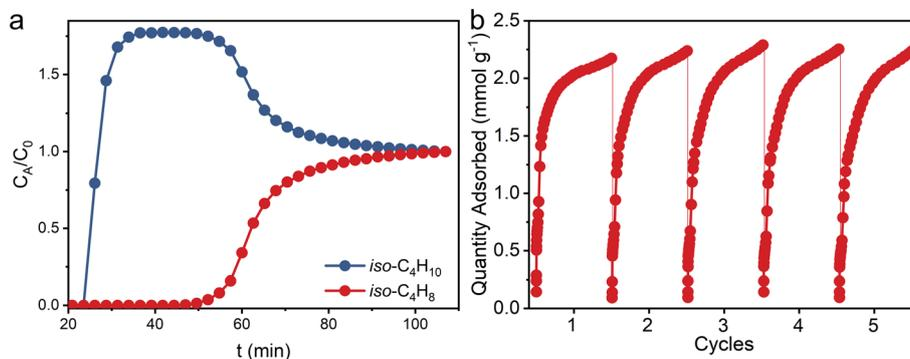
**Fig. 4** (a) Breakthrough experiment on ZU-603 using a gas mixture of iso-C<sub>4</sub>H<sub>8</sub>/iso-C<sub>4</sub>H<sub>10</sub> (50/50, v/v) with a mix gas flow rate of 0.8 mL min<sup>-1</sup> at 298 K and (b) cycling adsorption tests of iso-C<sub>4</sub>H<sub>8</sub> on ZU-603 at 298 K.
