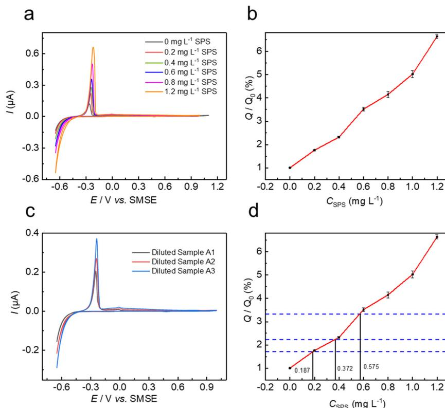
**Fig. 4** (a) Anodic stripping voltammograms obtained in VMS containing 500 mg L<sup>-1</sup> PEG, 4 mg L<sup>-1</sup> JGB and different SPS concentrations. (b) Calibration curve of the normalized anodic stripping charge of Cu as a function of SPS concentration. (c) Anodic stripping voltammograms of sample A1, sample A2 and sample A3. (d) SPS concentrations of the three samples derived from the calibration curve.
