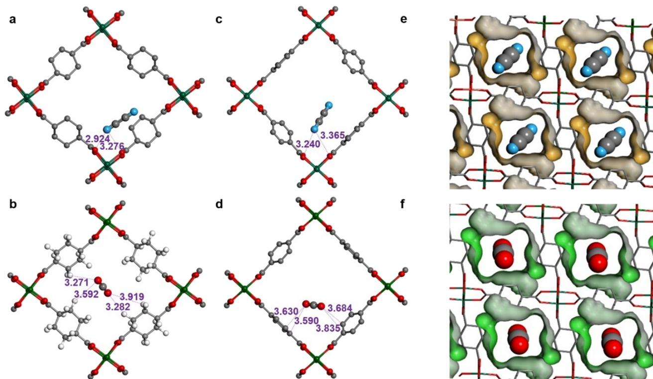
Fig. 5 Preferential binding sites of (a)  $C_2H_2$  and (b)  $CO_2$  in Cu(cyhdc) determined by GCMC simulations; preferential binding sites of (c)  $C_2H_2$  and (d)  $CO_2$  in Cu(bdc) determined by GCMC simulations; the unit of distance is Å. Cu, dark green; O, red; C, grey; H, pale grey. H atoms of (a), (c) and (d) are omitted for clarity. GCMC simulations of guest-inclusion structures for (e)  $C_2H_2$  loaded Cu(cyhdc) and (f)  $CO_2$  loaded Cu(cyhdc).
