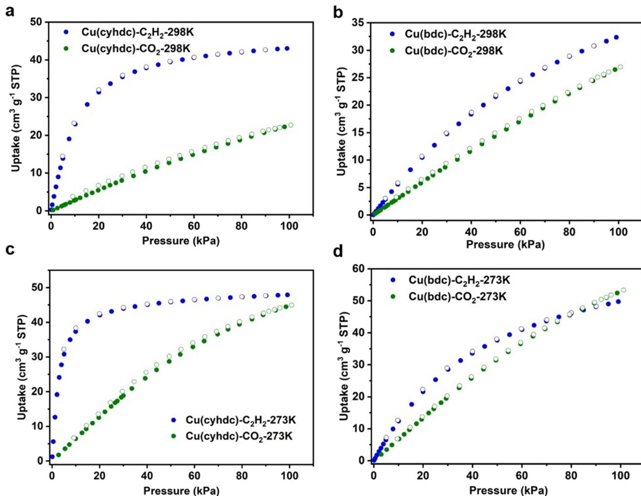
Fig. 3 C<sub>2</sub>H<sub>2</sub> and CO<sub>2</sub> adsorption isotherms of (a) Cu(cyhdc) and (b) Cu(bdc) at 298 K; (c) Cu(cyhdc) and (d) Cu(bdc) at 273 K.
